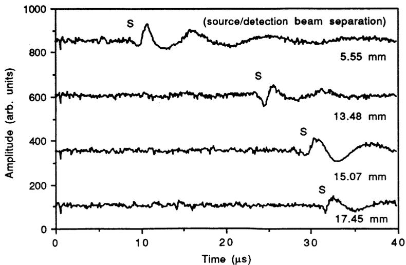
Fig. 6. Surface waves due to laser generated ultrasound for different separation distances between the detection and source lasers (S = Surface waves).
