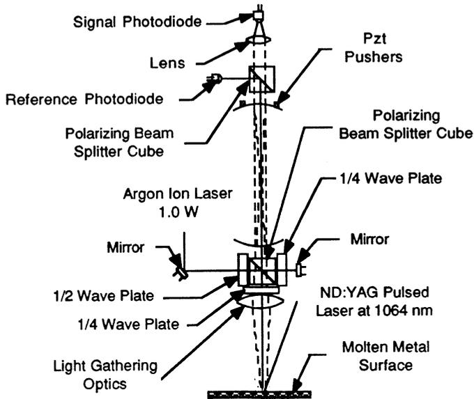
Fig. 2. Laser detection of ultrasound using a confocal Fabry-Perot interferometer.
