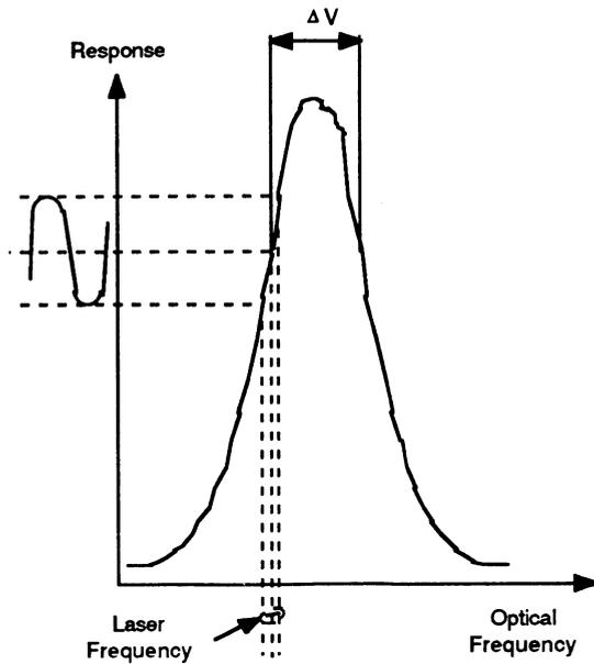
Fig. 1. The reflected light is demodulated by setting the laser frequency on the slope of one of the response peaks of the interferometer.
