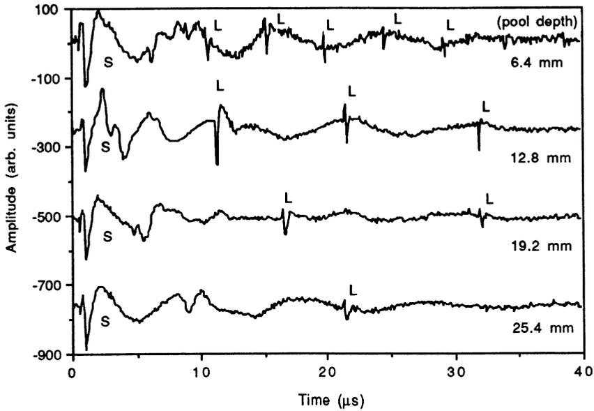
Fig. 4. Ultrasonic detection for four different pool depths (L = Longitudinal waves, S = Surface waves).
