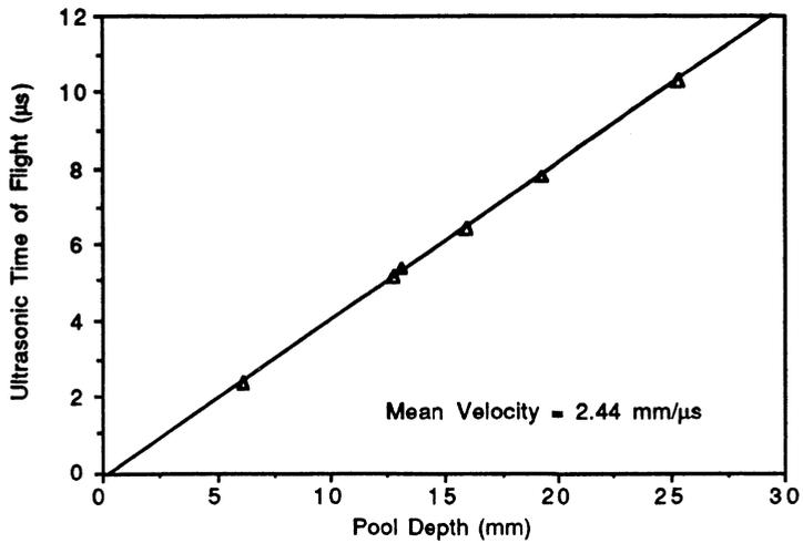
Fig. 5. Mean velocity calculation using six different pool depths.
