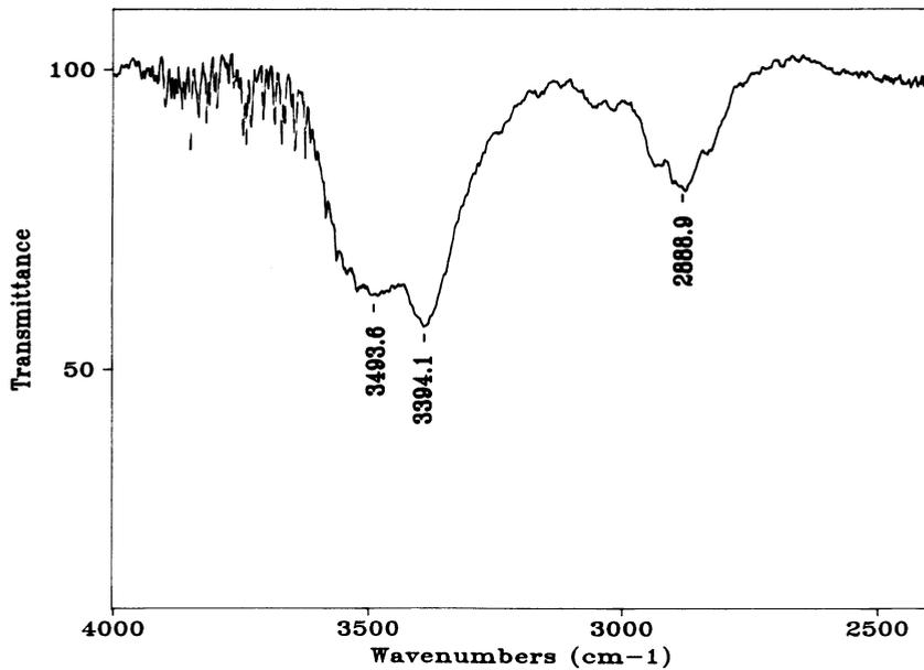
Fig. 7. Spectra of epoxy during cure at 350 °F.
