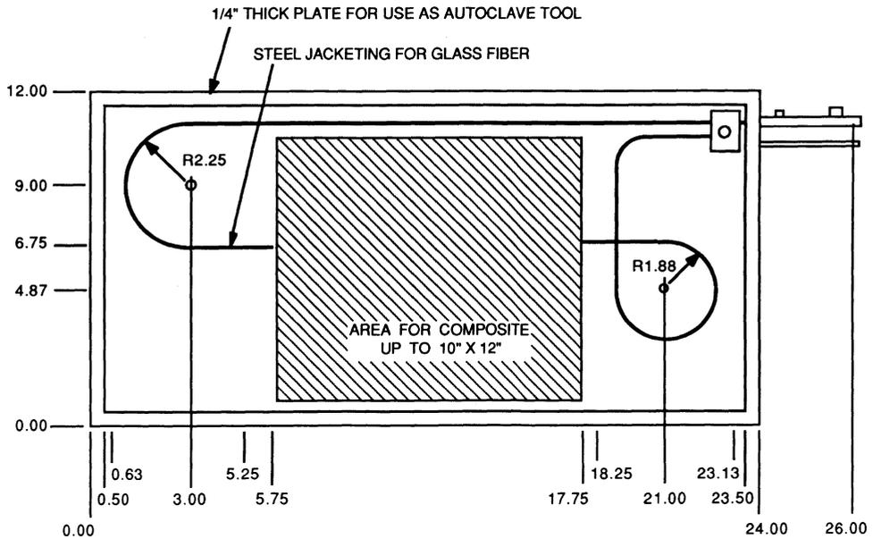
Fig. 3. Autoclave tool for laying up sensor fiber.
