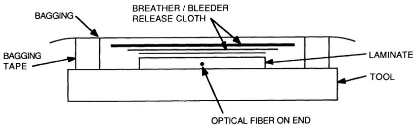
Fig. 4. Laying up of optical fiber in the laminate.
