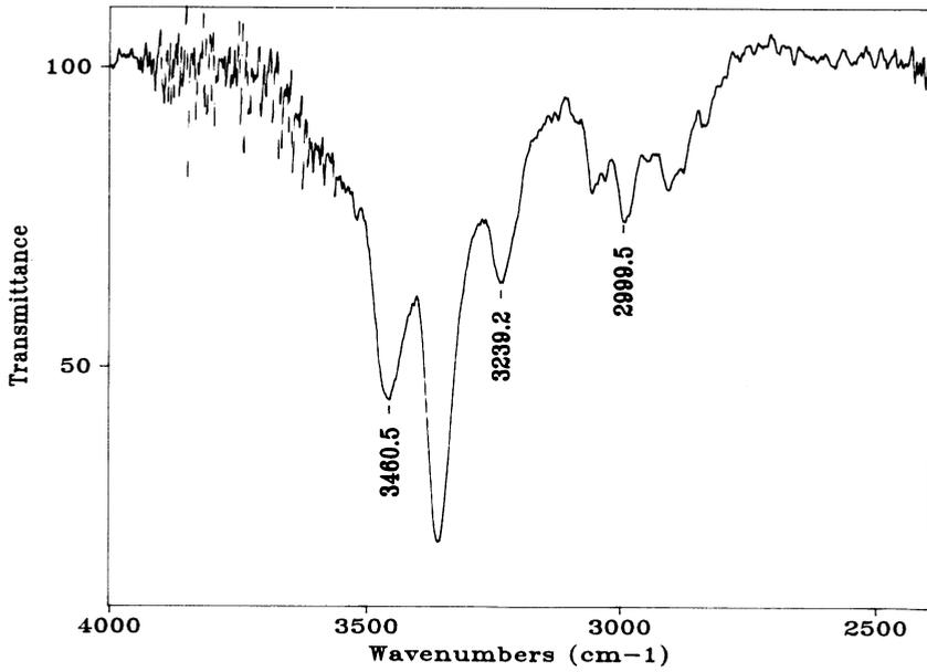
Fig. 6. Spectrum of epoxy at room temperature.
