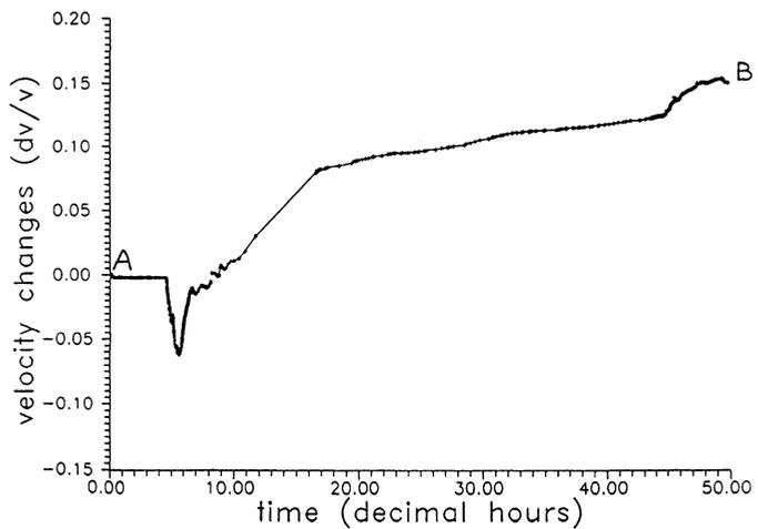
Fig.4 Velocity of ultrasound vs. time of processing. A: the starting point, tetragonal phase. B: finish point, orthorhombic phase.
