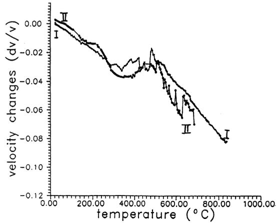
Fig.1 Velocity of ultrasound vs. temperature for heating from orthorhombic to tetragonal phase. Curve I-8MHz, curve II-3MHz data.
