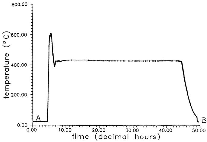
Fig. 3 Annealing schedule for the ultrasonic experiment.
