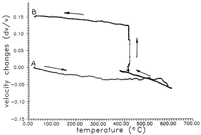
Fig.2 Velocity of ultrasound vs. temperature for processing from tetragonal to orthorhombic phase. Temperature-time dependence for the same experiment is shown in fig.3, the velocity-time dependence is presented on fig.4.
