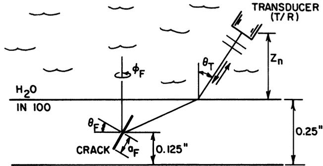
Fig. 3. Schematic representation of detection system and crack parameters used in simulation studies.
