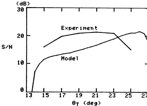
Fig. 7. Comparison between experimental and model simulated signal-to-noise versus transducer angle for fatigue crack in IN100 plate.
