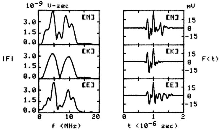
Fig. 1. Comparison of theoretical and experimental frequency and time domain signals from a circular crack ( $a_F=0.022\text{cm}$ ) in thermoplastic sample at  $30^\circ$  illumination angle (M=MOOT, K=Kirchhoff, E=Experiment).
