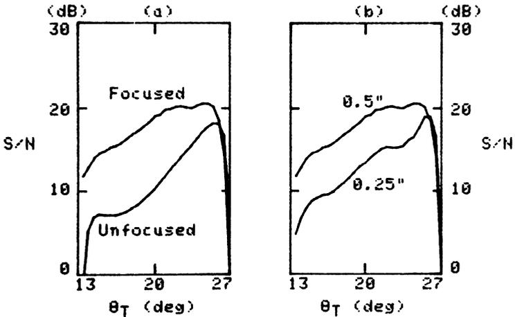
Fig. 6. Example of improved detectability using focussed transducers. a) signal-to-noise versus transducer angle for unfocussed and unfocussed probe. b) signal-to-noise versus transducer angle for focussed probes of different radii.
