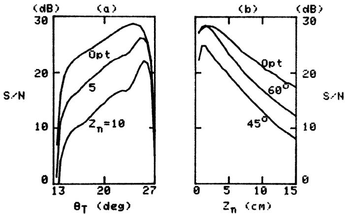
Fig. 4. Example of detection system design analysis. a) signal-to-noise versus transducer angle at various distances to sample. b) signal-to-noise versus separation distance at various transducer angles.
