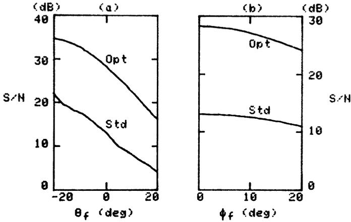
Fig. 5. Example of improved detectability using improved system configuration. a) signal-to-noise versus crack inclination. b) signal-to-noise versus crack azimuthal angle.
