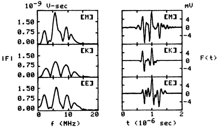
Fig. 2. Comparison of theoretical and experimental frequency and time domain signals from a circular crack ( $a_F=0.022\text{cm}$ ) in thermoplastic sample at  $60^\circ$  illumination angle (M=MOOT, K=Kirchhoff, E=Experiment).
