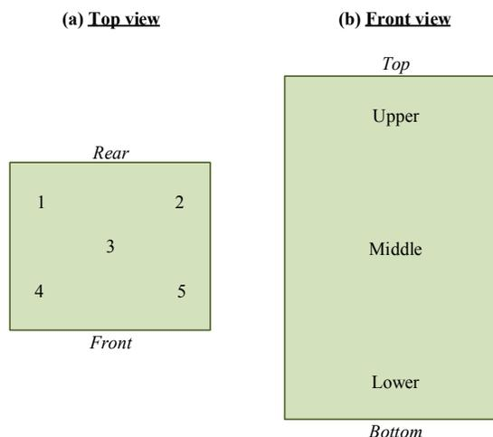
Figure 1. Static pressure sampling locations and heights: (a) top view showing the five sampling locations per height in the chamber and (b) front view showing the three sampling heights (upper, middle, and lower).
