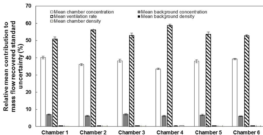
**Figure 8. Relative mean contribution to mass flow recovered standard uncertainty averaged for all replicates. Error bars represent standard deviations obtained by replicates. Other parameters are omitted for clarity and had <3% contribution. Major contributions from ventilation rate and concentration measurement were consistent across all the six chambers.**
