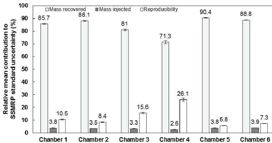
Figure 10. Mean relative contribution to steady-state mass recovery percent (SSMRP) standard uncertainty for all replicates. Error bars represent standard deviations for replicates ( $n = 8$ ). Mass recovered had the greatest contribution, while the contribution of reproducibility was positively correlated with its magnitude.
