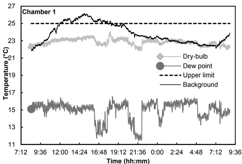
**Figure 5. Example of temperature measurement over approximately 23 h for chamber 1 and the background. All chambers were maintained within the desired temperature range (upper limit of 25°C shown in figure) despite exceeding background conditions, and no condensation formed inside the chambers.**
