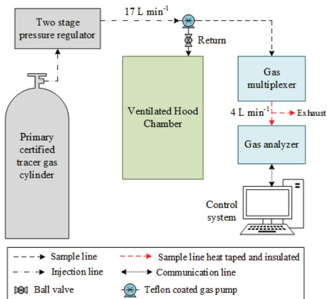
Figure 2. Configuration of gas sampling subsystem integrity test for one chamber. The sampling line was disconnected from the sampling port at the top of the chamber and connected to the outlet of a tracer gas cylinder. FASMS, TECS, and other GSS components are omitted for clarity. The same procedure and configuration were used for each of the six chambers.
