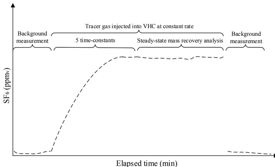
Figure 4. The system was considered to be at steady-state after five system time constants. The recovery test procedure measured background concentration first, allowed the chamber to reach steady-state, and concluded with additional background measurement.
