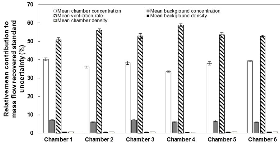
Figure 9. Relative mean contribution to mass flow injected standard uncertainty averaged for all replicates. Standard deviations obtained by replicates were much less than 1%. Injected flow contributed approximately 91% to mass flow injected standard uncertainty.
