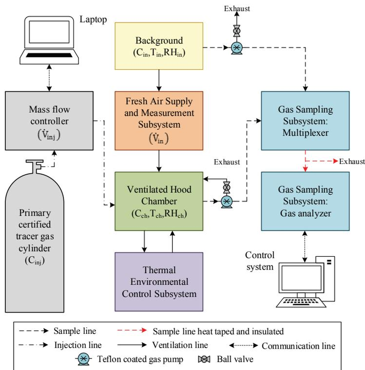
Figure 3. Experimental setup for steady-state mass recovery test in one chamber. Tracer gas ( $C_{inj}$ ) was supplied at a constant volumetric flow rate ( $\dot{V}_{inj}$ ) from a mass flow controller. Mass recovered was determined from temperature ( $T_{in}$ ,  $T_{ch}$ ), relative humidity ( $RH_{in}$ ,  $RH_{ch}$ ), gas concentration ( $C_{in}$ ,  $C_{ch}$ ), and ventilation rate ( $\dot{V}_{in}$ ) measurements in REMS.
