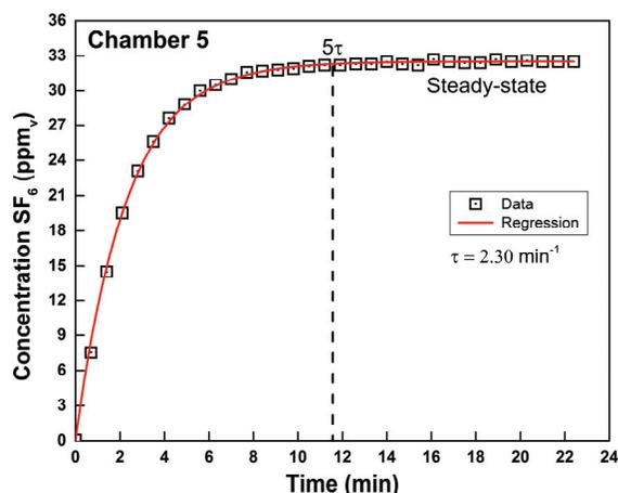
**Figure 7. Example of the nonlinear regression steady-state analysis for one chamber. The solid line is the nonlinear regression (eq. 2) fitted to the measured concentrations (data). Five time constants ( $5\tau$ ) were used as a conservative estimate for determining the time to steady-state ( $< 14$  min for all chambers).**
