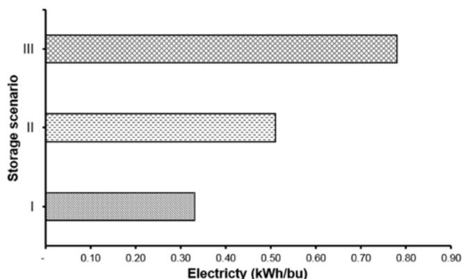
Figure 6 Electricity usage (kW h bu<sup>-1</sup>) three different scenario for small and middle-sized farmers
