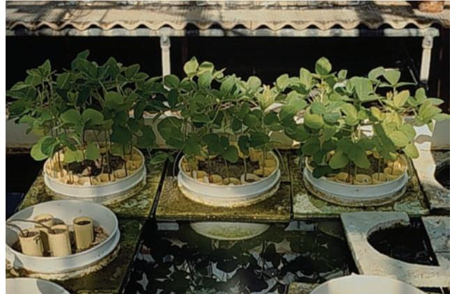
Temperature-controlled water bath in greenhouse in which HG type tests are conducted. (Greg Tylka)
