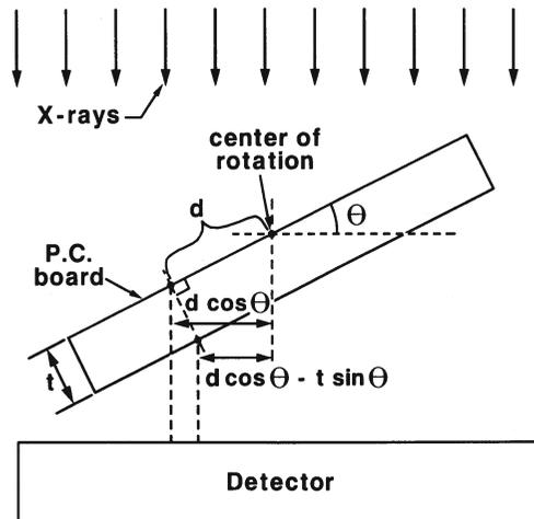
Fig. 1. Geometry for digital stereo radiography measurements.
