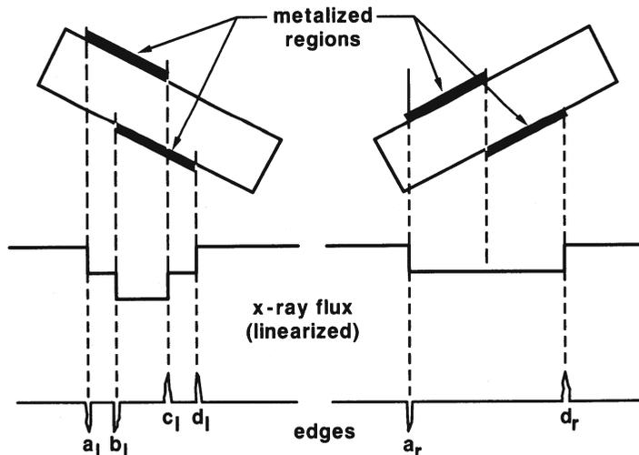
Fig. 2. Demonstration of how two edges can coincide to cancel each other.
