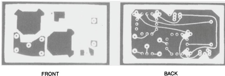
Fig. 5. Front and back images determined from the stereo pair of radiographs in Fig. 4 using the algorithm outlined in Fig. 3.
