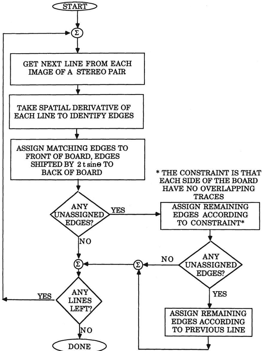
Fig. 3. Flowchart for digital stereo radiography algorithm.
