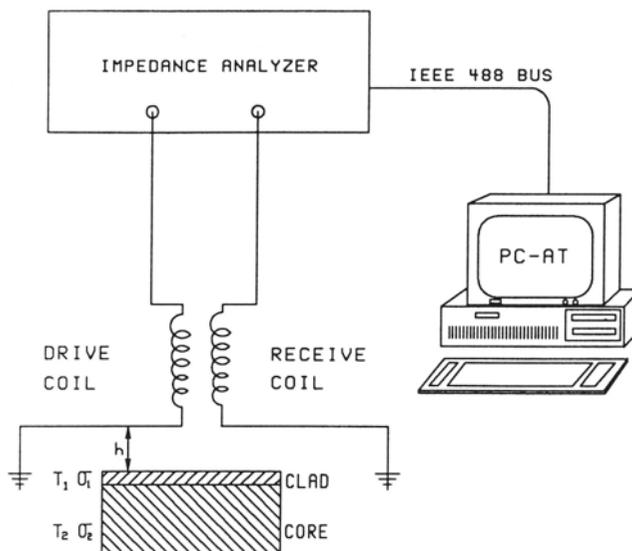
Fig. 2. Diagram for instrumentation used in measurements.
