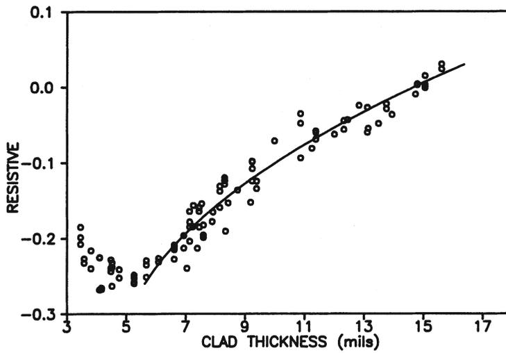
Fig. 4. Clad thickness relationship for resistive change against thickness at 100 kHz.
