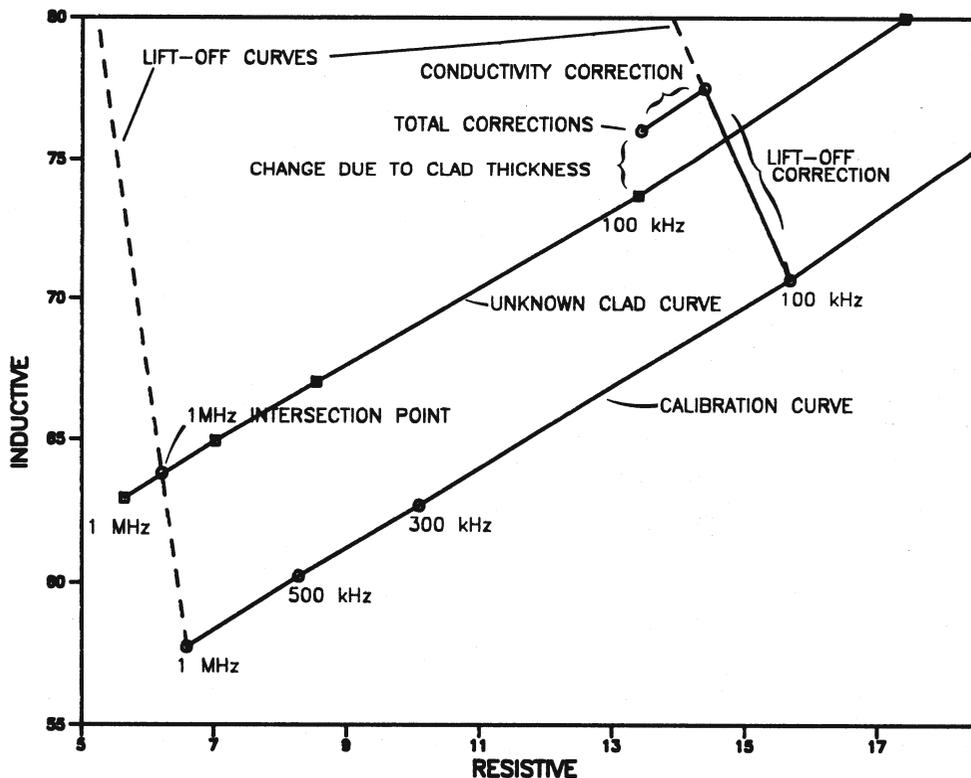
Fig. 3. Correction technique for measurement of clad sample having an unknown thickness.
