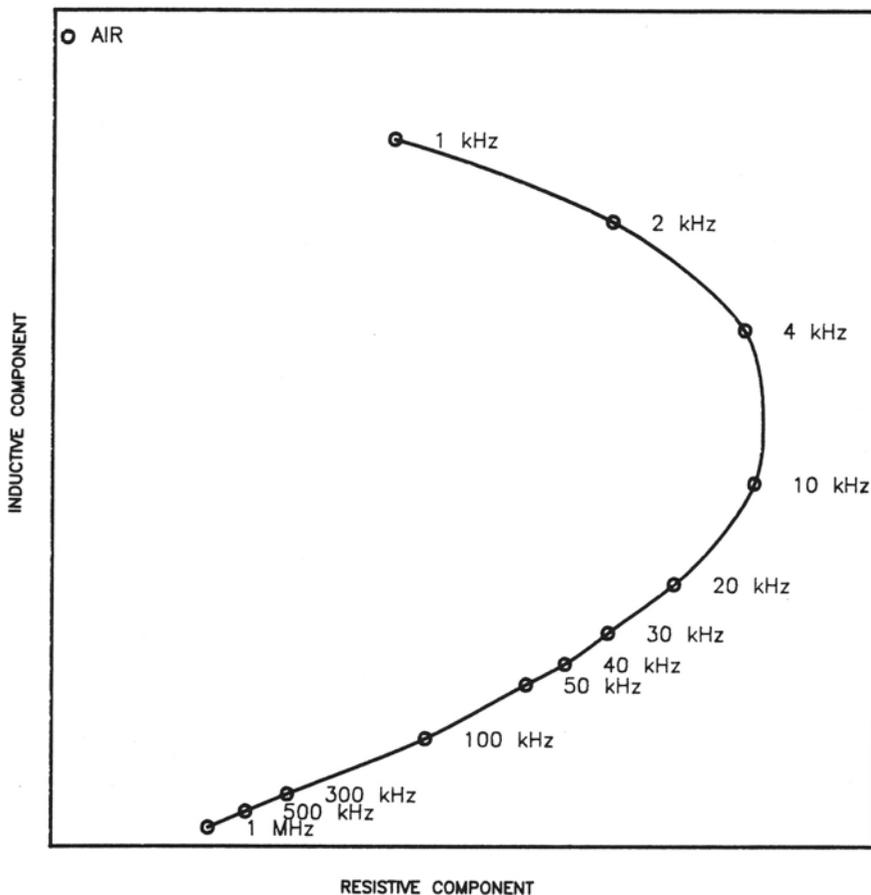
Fig. 1. Impedance curve for the measurement coil configuration.
