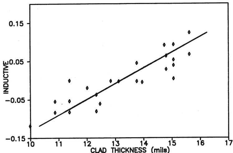
Fig. 6. Clad thickness relationship for inductive change against thickness at 30 kHz.
