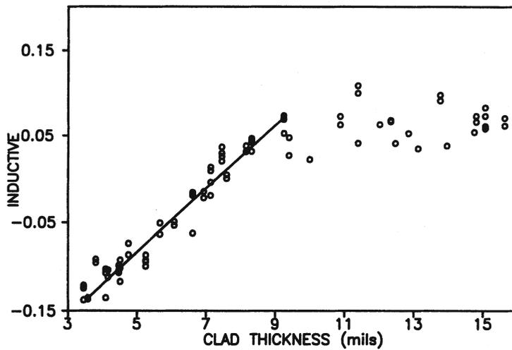
Fig. 5. Clad thickness relationship for inductive change against thickness at 100 kHz.
