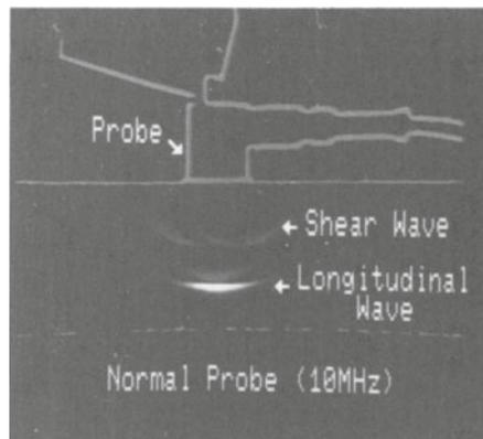
Fig. 4 Generation of longitudinal wave and shear wave from a 10 MHz normal probe
