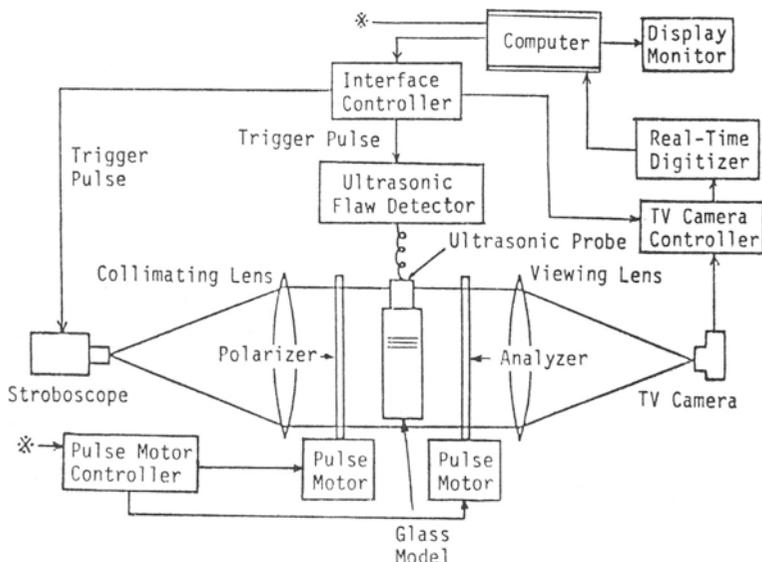
Fig. 1 Diagram of Ultrasonic Wave Visualization System
