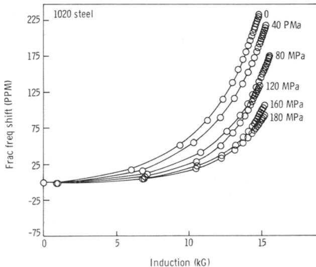
Fig. 1.  $\Delta f(B)/f$  curves obtained for the 1020 steel sample under uniaxial tension.
