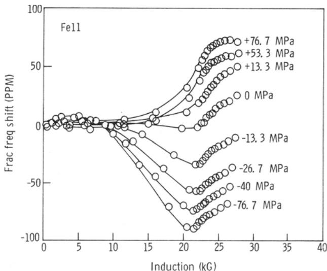
Fig. 7.  $\Delta f(B)/f$  curves obtained for another pure iron sample prepared under identical conditions.
