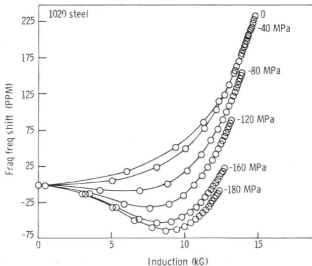
Fig. 2.  $\Delta f(B)/f$  curves obtained for the 1020 steel sample under uniaxial compression.
