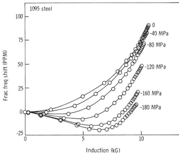
Fig. 5.  $\Delta f(B)/f$  curves obtained for the 1095 steel sample under uniaxial compression.
