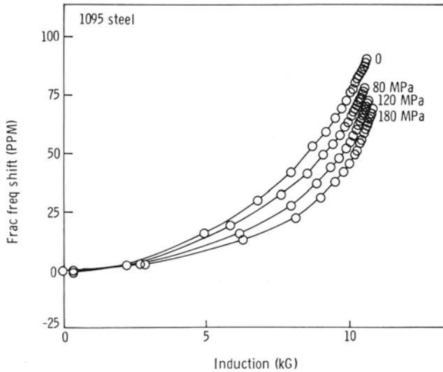
Fig. 4.  $\Delta f(B)/f$  curves obtained for the 1095 steel sample under uniaxial tension.
