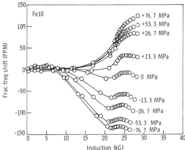
Fig. 6.  $\Delta f(B)/f$  curves obtained for a pure iron sample by applying the magnetic field parallel to the stress axis and propagating compressional waves through the field axis.
