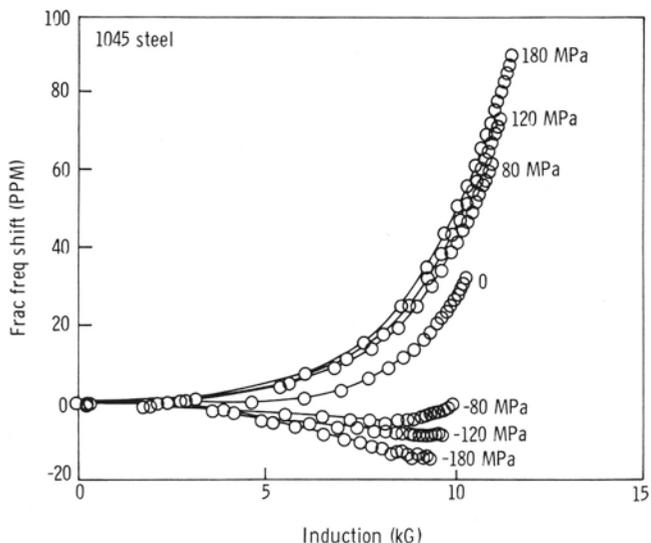
Fig. 3.  $\Delta f(B)/f$  curves obtained for the 1045 steel sample.
