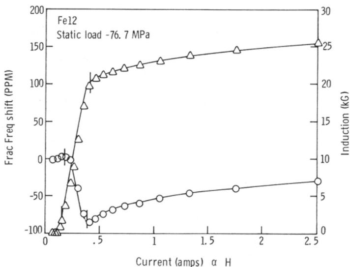
Fig. 8.  $\Delta f(B)/f$  and magnetization curves obtained for a pure iron sample.
