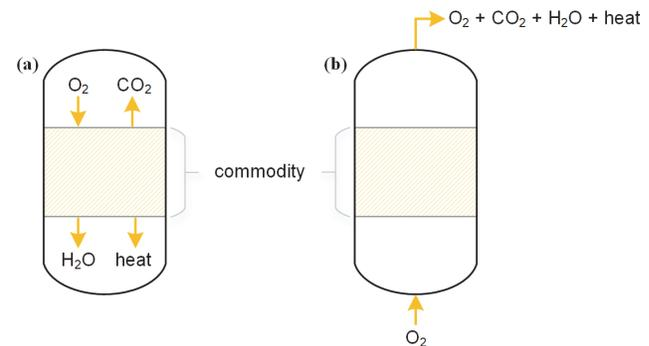
Figure 1. Schematic of (a) static and (b) dynamic grain respiration measurement systems (S-GRMS and D-GRMS).
