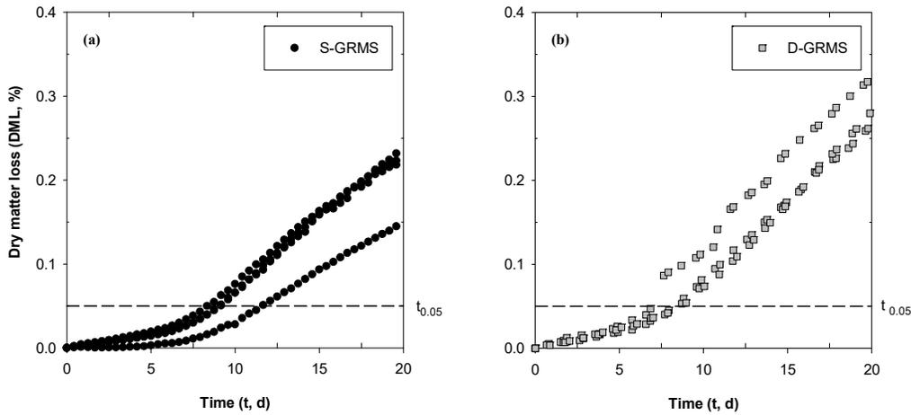
Figure 7. Dry matter loss estimates (DML, %) over time ( $t$ , d) of 18% moisture content soybeans at 30°C in (a) static and (b) dynamic grain respiration measurement systems (S-GRMS and D-GRMS).
