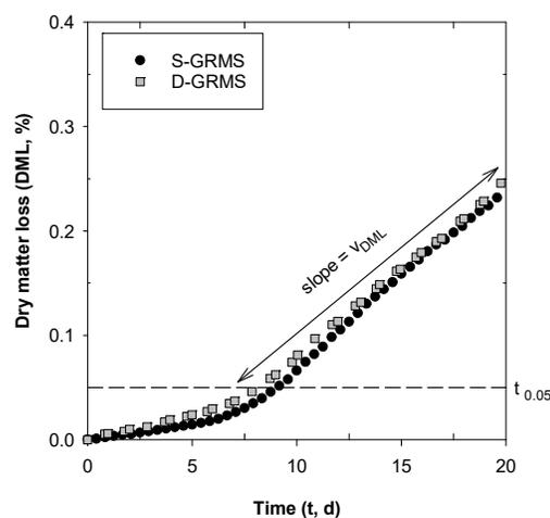
Figure 6. Dry matter loss rates ( $v_{DML}$ ,  $\% \text{ d}^{-1}$ ) in static and dynamic grain respiration measurement systems (S-GRMS and D-GRMS) were estimated as the slope of the linear increase after  $\text{DML} = 0.05\%$ . This threshold was considered the lag period of a respiration test.
