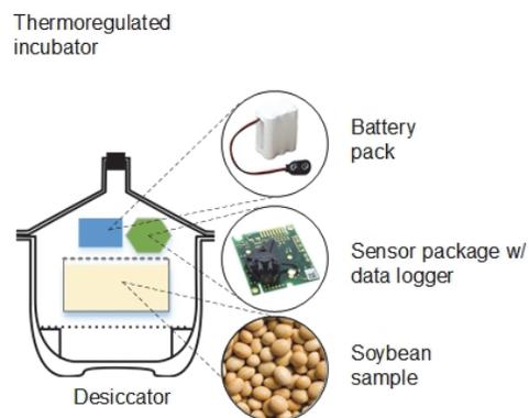
Figure 3. Each static grain respiration measurement system (S-GRMS) included a 10 L desiccator as the respiration chamber capable of holding a 500 g soybean sample and a battery-operated sensor package to monitor temperature, relative humidity, and  $C_{CO_2}$  inside the chamber. The temperature of the S-GRMS unit was controlled over time by placing it inside a thermoregulated incubator.
