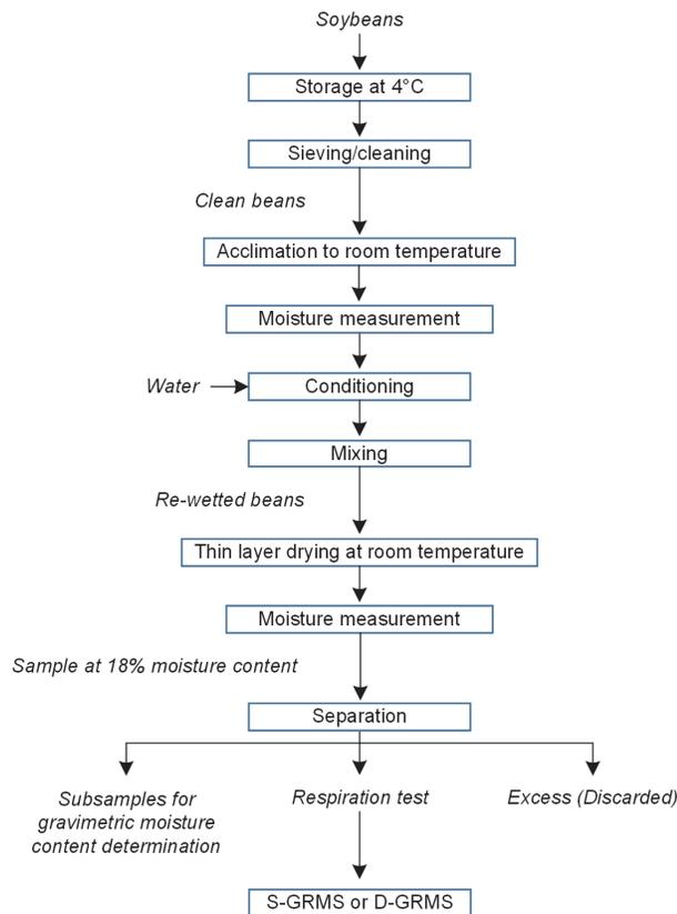
Figure 2. Soybean sample preparation for S-GRMS and D-GRMS.
