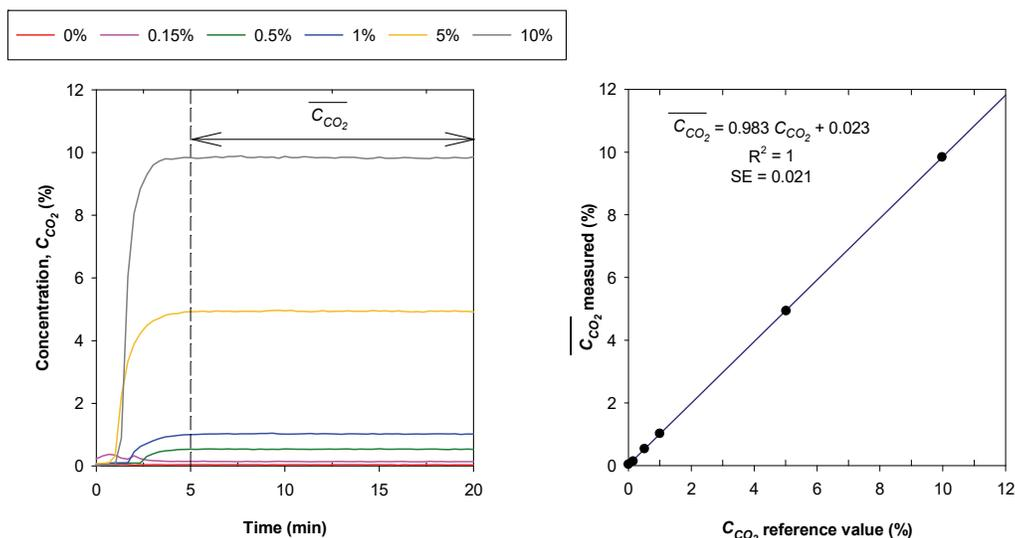
Figure 4. Carbon dioxide concentrations over time and an example regression for one sensor package.
