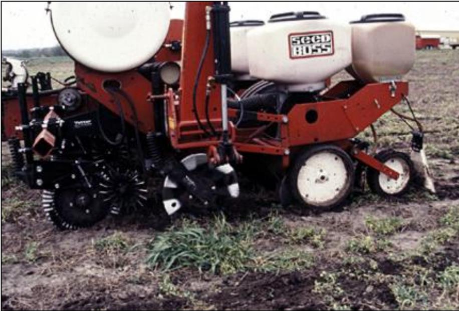
*Planter seed-opener, depth wheels, and closing system should be adjusted to ensure proper seed depth and adequate seed-soil contact without overly compacting soil.*
