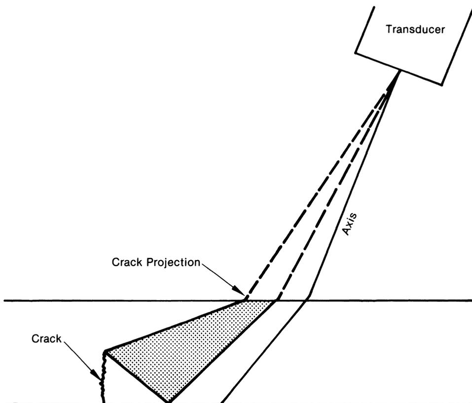
Fig. 2. Geometry of the setup used in model calculations and experiments.
