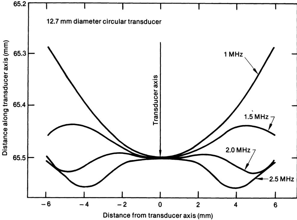
Fig. 3. Approximate wavefront shapes at four different frequency components.
