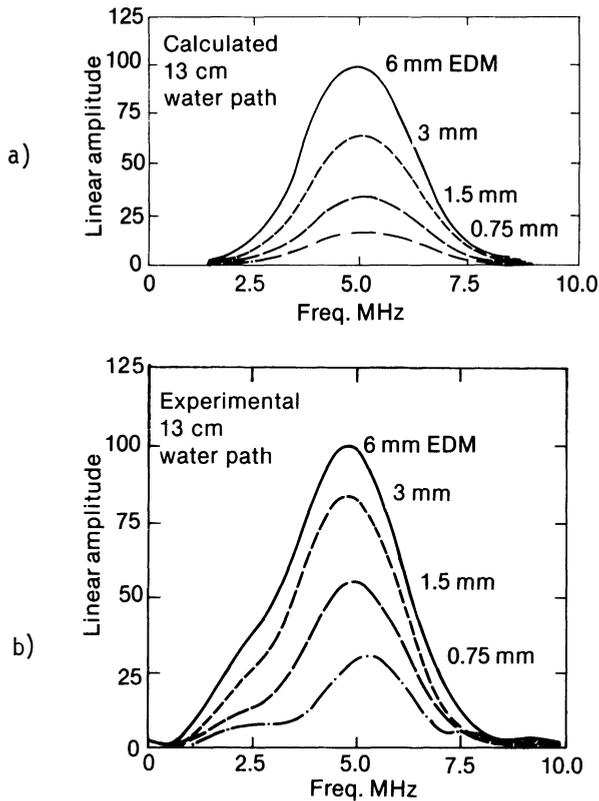
Fig. 5. Calculated (a) and measured (b) spectra from four EDM notches of different sizes. All are the maximum amplitude reflection.
