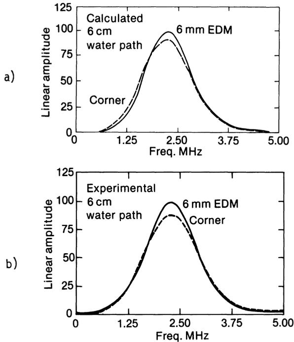
Fig. 6. Calculated (a) and measured (b) spectra from a 6-mm EDM notch and a machined corner in the same bar representing a through-wall crack.
