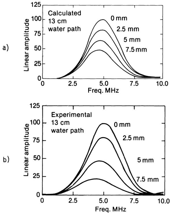
Fig. 4. Calculated (a) and measured (b) spectra from a 6-mm EDM notch at four transducer positions. Maximum amplitude is at 0 mm.
