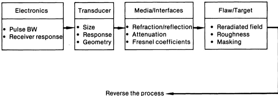
Fig. 1. Elements of the transducer field and flaw interaction.
