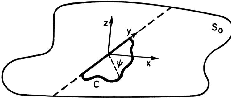
Fig. 1 Geometry of the cracks considered in this paper.  $S_0$  is the infinite plane boundary between the linear isotropic and homogeneous elastic medium which occupies the half-space  $z < 0$ . The crack  $C$  can be buried or can break the  $xy$  plane  $S_0$ ; it lies in a plane which contains the  $y$ -axis and makes an angle  $\psi$  with the  $x$ -axis. For the sake of algebraic simplicity in the present work we take  $\psi = 90^\circ$ ; i.e.  $C$  lies in the  $yz$  plane.
