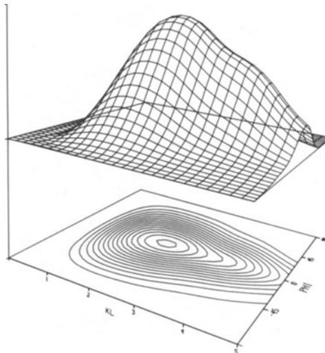
Figure 8. Rayleigh backscattering amplitude for a  $7 \times 7$  triangular crack buried at  $d_0 = 10.5a$ . As expected, the amplitude decreases rapidly when the wavelength becomes less than the burial depth.
