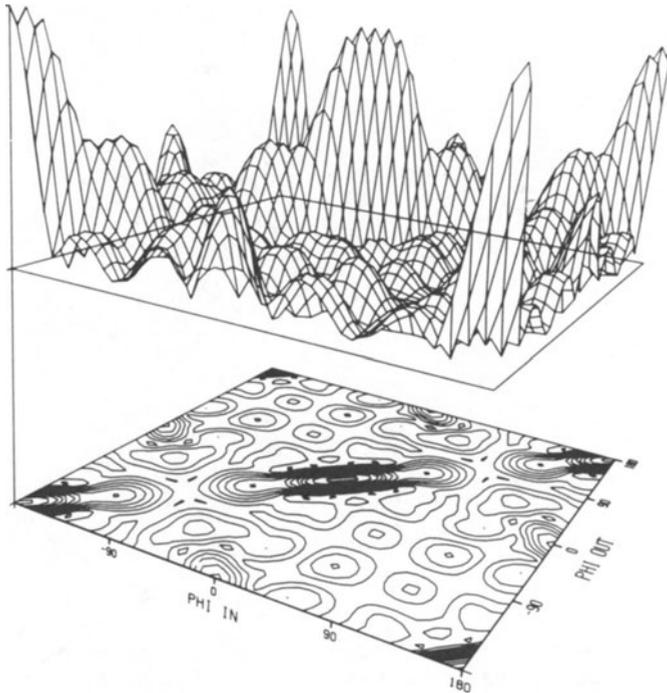
Figure 4. Angular dependence of the modulus of the Rayleigh surface wave scattering amplitude, as a function of azimuths for a rectangular ( $9 \times 6$ ) surface-breaking crack with  $k_s L = 8$ . This function is symmetric about the main diagonal and the antidiagonal and it has a pronounced ridge along the specular reflection line.
