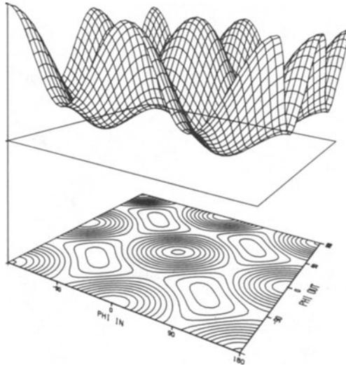
Figure 3. Angular dependence of the modulus of the Rayleigh surface wave scattering amplitude, as a function of azimuths  $\phi_{in}$  and  $\phi_{out}$ , for a square ( $7 \times 7$ ) surface-breaking crack with  $kL = 0.2$ . The dependence of this amplitude on the size and shape and burial depth is describable by just 2 parameters in this long wavelength situation. The shape of this surface for a triangular surface-breaking crack is nearly indistinguishable; it has the same symmetries.
