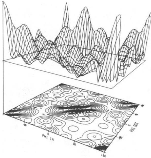
Figure 5. Scattering amplitude at  $k_s L = 8$  from a  $9 \times 6$  triangular surface-breaking crack. The specular ridge is pronounced, and symmetry about the main diagonal has disappeared.
