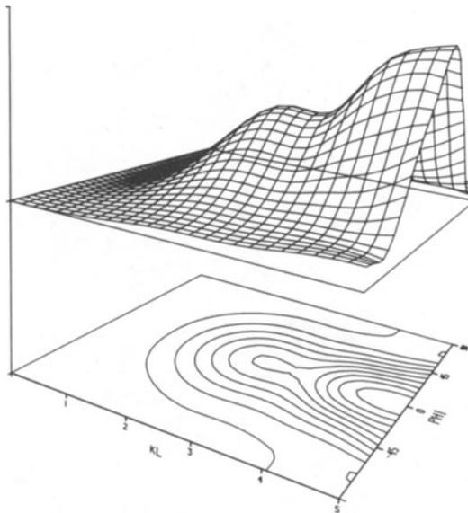
Figure 6. Modulus of the backscattered amplitude from a  $12 \times 5$  rectangle for  $0 < k_s L \leq 5$ . At low frequencies the amplitude rises like  $(k_s L)^{5/2}$ .
