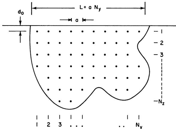
Figure 2. The positions of the centers of the gaussian localized functions are chosen in a square array whose boundaries approximate the crack edges.  $d_0$ , the depth of the topmost line of centers needed to simulate a surface-breaking crack, is one of the parameters which must be determined. This crack has  $\psi = 90^\circ$ ; it lies in the  $yz$  plane.
