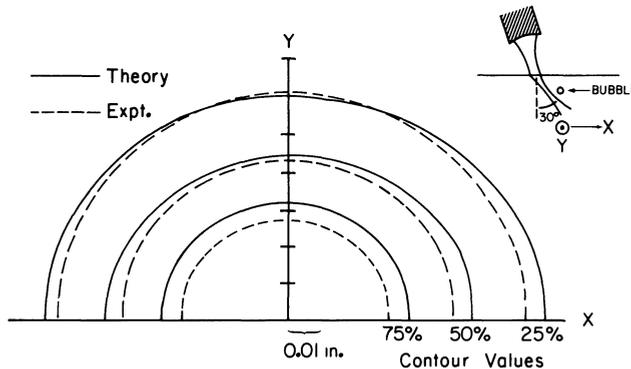
Fig. 5. Comparison of measured and predicted response of a scanned,  $30^\circ$  angle longitudinal scan. The transducer was a 5 MHz, 0.5 in. (1.27 cm) diameter, 4 in. (10 cm) focal length probe. The flaw was a  $300\mu\text{m}$  diameter pore in glass, at a depth of about 1 cm. Transducer height was adjusted to place the pore in the focal plane.
