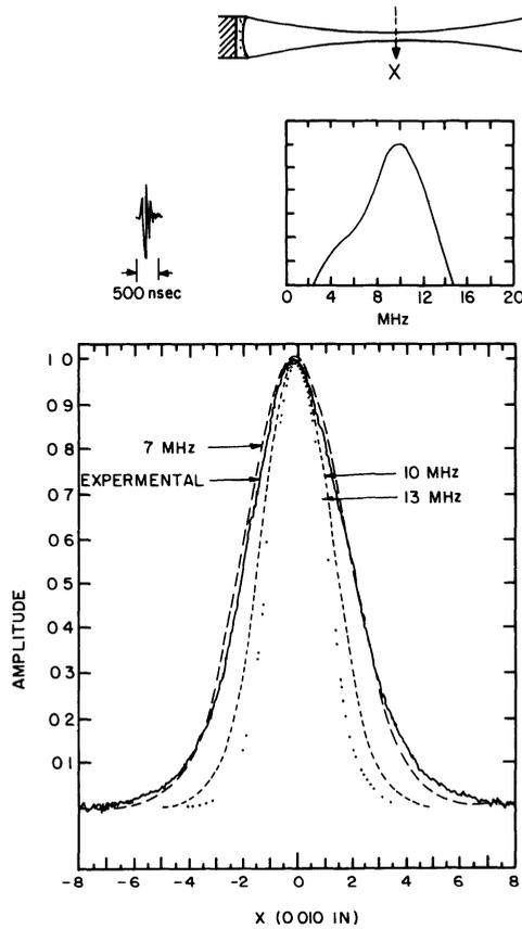
Fig. 3. Comparison of Gaussian fit to measured transverse beam patterns in the focal plane of a 10 MHz, 1.9cm diameter, 10.16cm focal length commercial probe. The time and spectral responses of the probe are shown at the top. The solid curve at the bottom is the variation of the peak pulse-echo response from a small spherical reflector while the broken curves are monochromatic expectations at three frequencies in the pass band.
