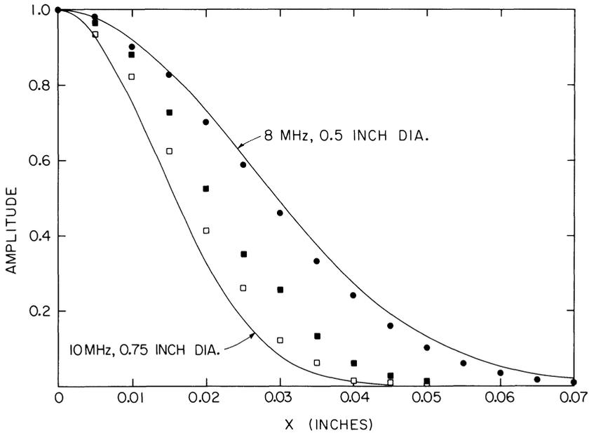
Fig. 4. Monochromatic radiation pattern in the focal plane of two commercial probes with 10.16cm nominal focal length. The solid lines are theoretical predictions and points are measured. A beam asymmetry in the 0.75 inch probe is indicated by two sets of data.
