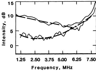
Comparison of Scattering from Grains and IGSCC, MHz
