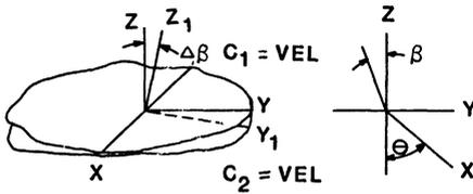
Figure 8. Correction for Surface Orientation
