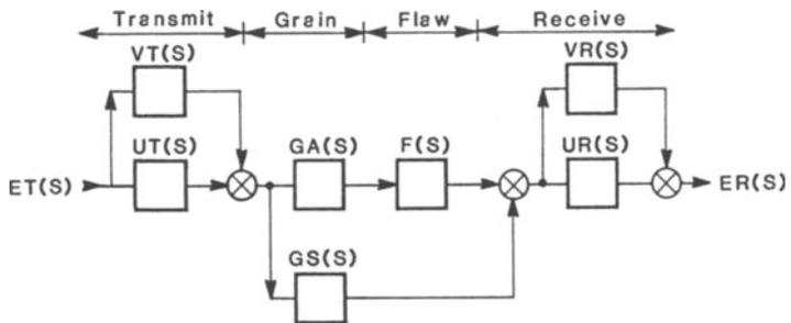
Figure 2. Ultrasonic Instrumentation Model
