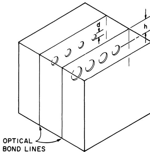
Fig. 6. Schematic diagram of fused quartz block with seeded, subsurface, vertical cracks.
