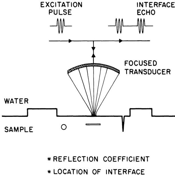
Fig. 1. Schematic diagram showing the principle of operation of the acoustic microscope. The interface echo is shown to be a function of the local reflection coefficient, and the location of the reflector.
