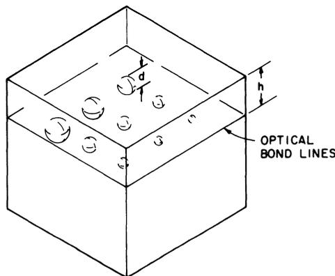
Fig. 4. Schematic diagram of fused quartz block with seeded, subsurface, spherical voids.
