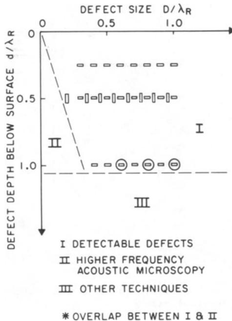
Fig. 8. Graph showing subsurface defect detection limit as a function of feature size (diameter) and depth.
