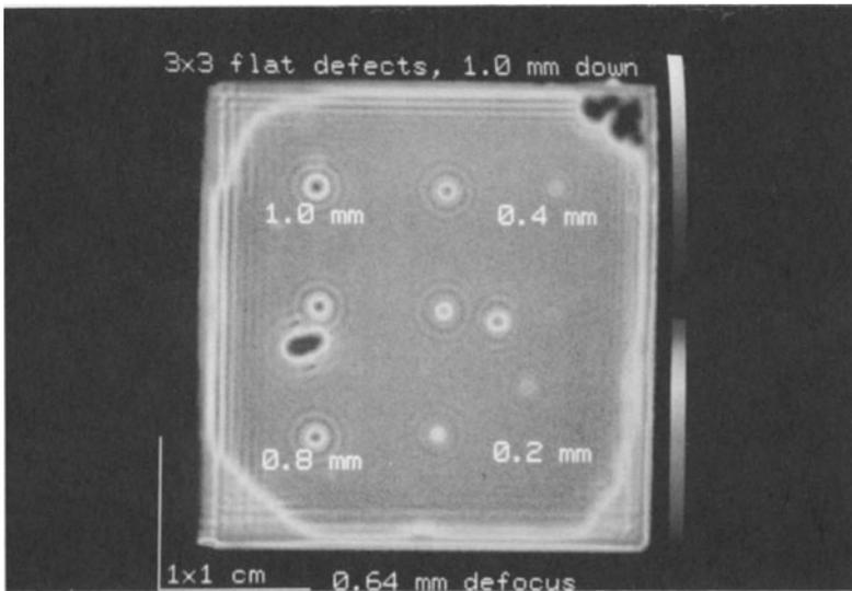
Fig. 3. Acoustic microscope picture of the sample of Fig. 2. The cracks are 1 mm below the surface, and the microscope is defocused by 0.64 mm. The diameters of the cracks vary from 0.2 mm to 1.0 mm.
