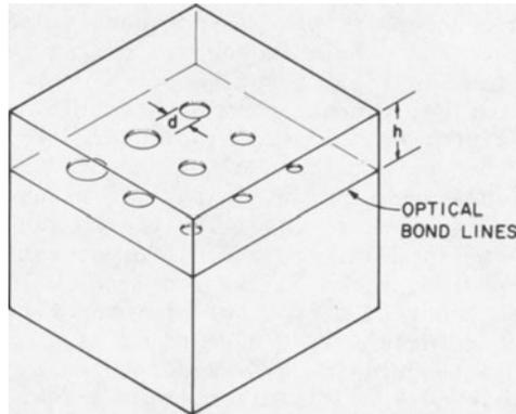
Fig. 2. Schematic diagram of fused quartz block with seeded, sub-surface, horizontal cracks.
