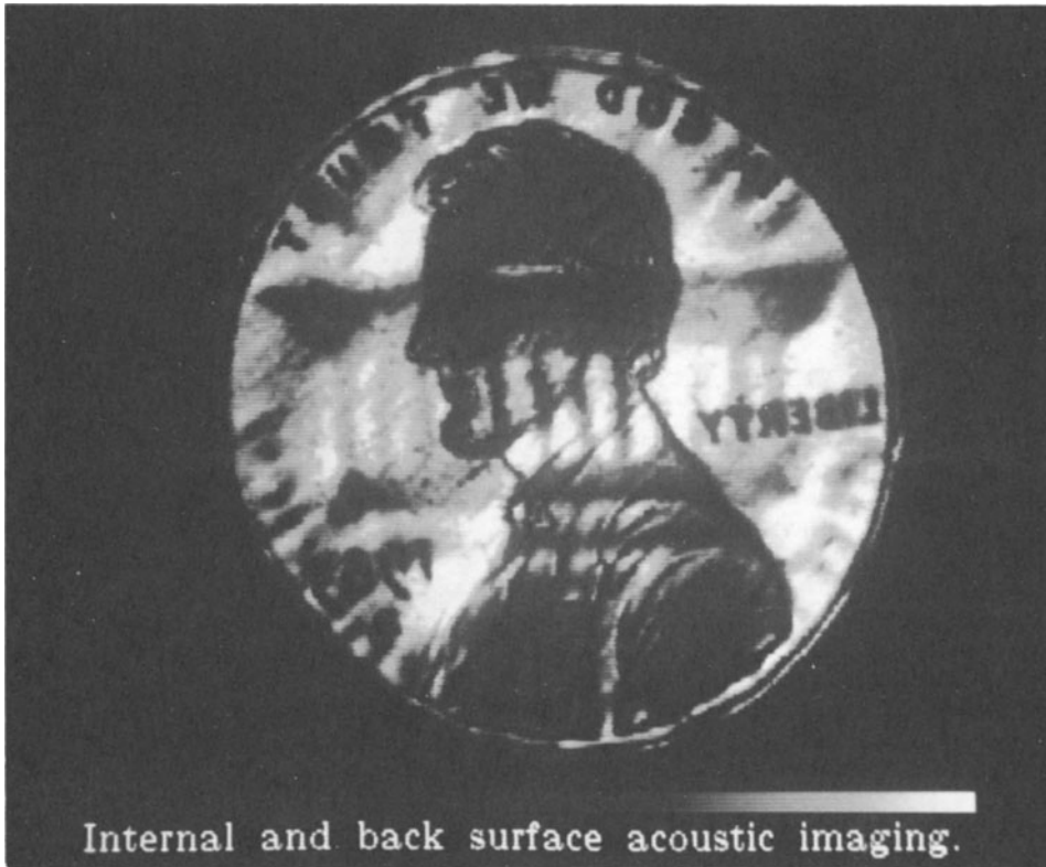
Figure 1. Images of modified Lincoln penny; front face (Memorial was machined to remove all copper material, leaving flat zinc face; raster-scanned acoustic image of front face, focused at plane of back face (head).
