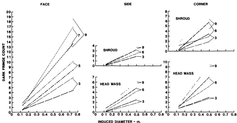
Fig. 6. Dark fringe count vs induced debond diameter; indicated debond locations. The parameter is vacuum level in inches of Mercury.
