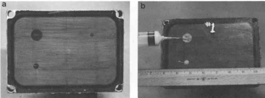
Fig. 4. Molded Head Mass Subassemblies With Induced Debonds
