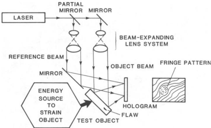
Fig. 1. Diagram of Holographic Inspection Technique
