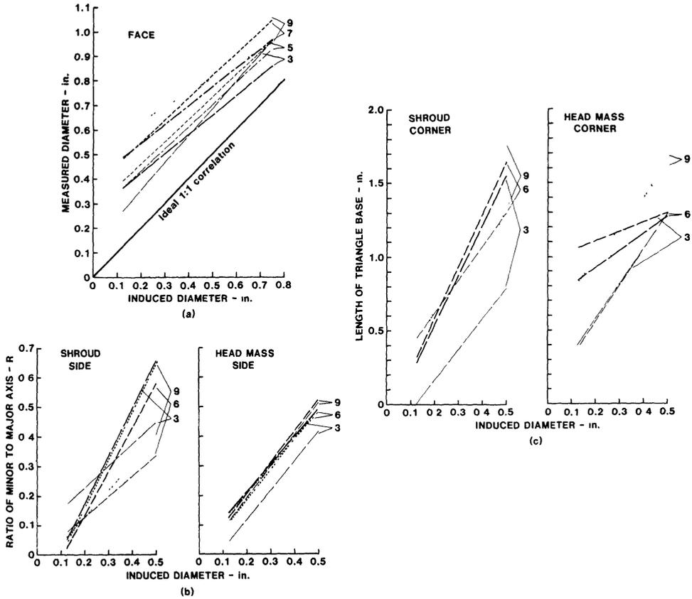
Fig. 7. Bullseye measurements vs induced debond diameter. (a) Bullseye diameter, face debonds, Location (A). (b) Ratio of bullseye axis lengths, annulus debonds, Locations (B) and (C). (c) Length of triangular bullseye base, corner debonds, Locations (D) and (E). The parameter is vacuum level in inches of Mercury.
