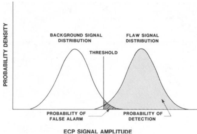
Fig. 3. Schematic illustration of probability density functions for signals and background noise.
