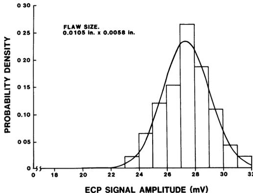
Fig. 8. Flaw signal probability density function for a 0.0105 in. x 0.0058 in. flaw with 0.008 in. scan track spacing.
