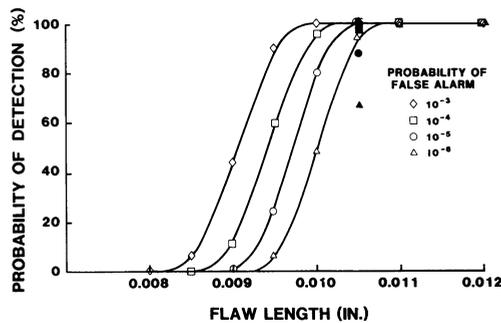
Fig. 9. Probability of detection detail for 0.008 in. scan track spacing. Open symbols are based on the approximation discussed in the text; solid symbols are based on actual experimental data.
