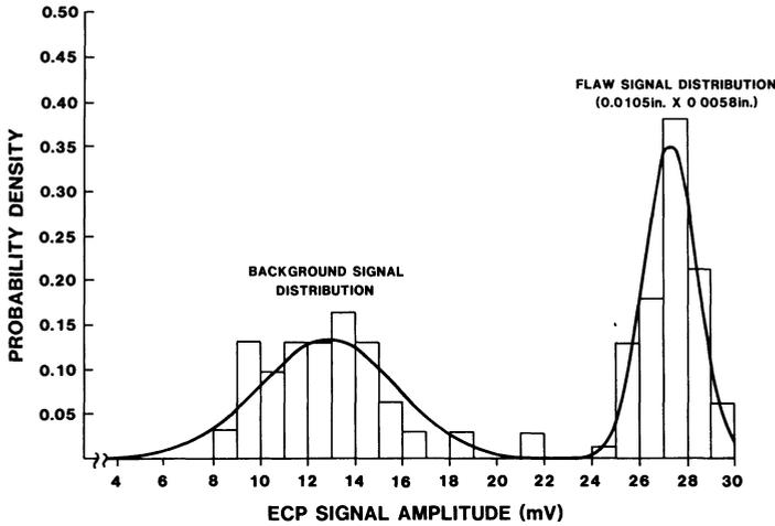
Fig. 5. Signal and background probability density functions for blade slots.
