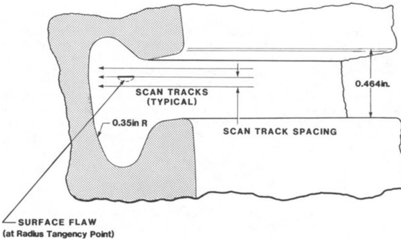
Fig. 2. Scan configuration for blade slots.
