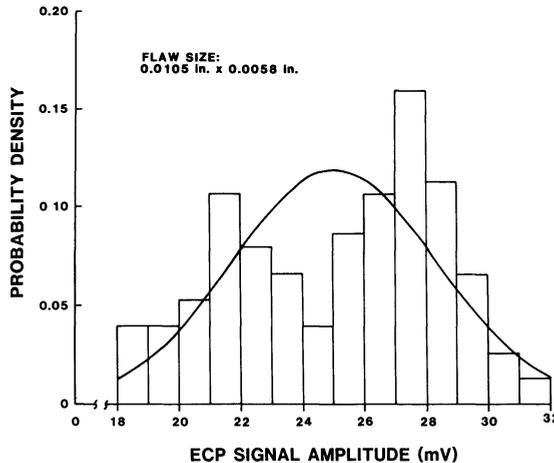
Fig. 6. Flaw signal probability density function for a 0.0105 in. x 0.0058 in. flaw with 0.014 in. scan track spacing.
