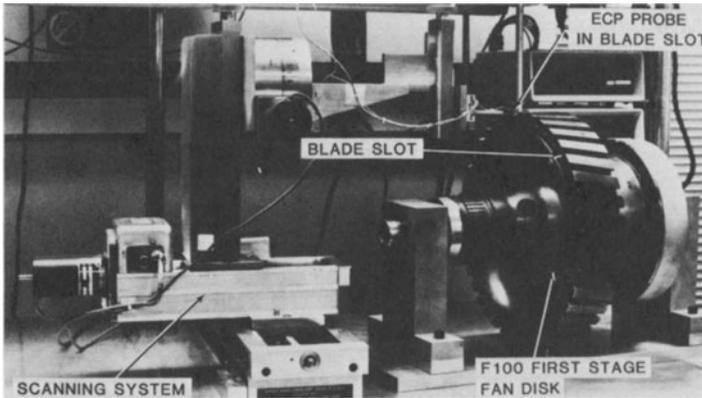
Fig. 1. ECP laboratory breadboard scanning system with F-100 first stage fan disk in place.
