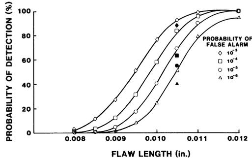
Fig. 10. Probability of detection detail for 0.014 in. scan track spacing. Open symbols are based on the approximation discussed in the text; solid symbols are based on actual experimental data.
