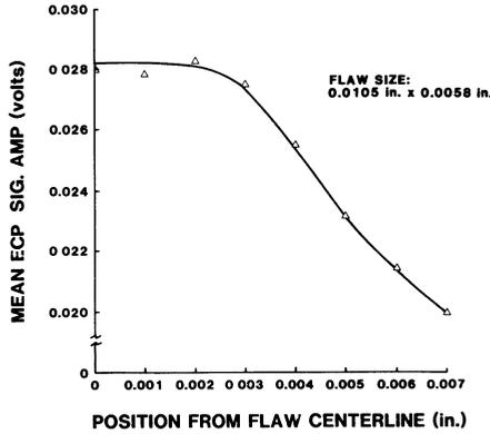
Fig. 7. Mean signal amplitude for a 0.0105 in. x 0.0058 in. flaw as a function of flaw-to-scan track spacing.
