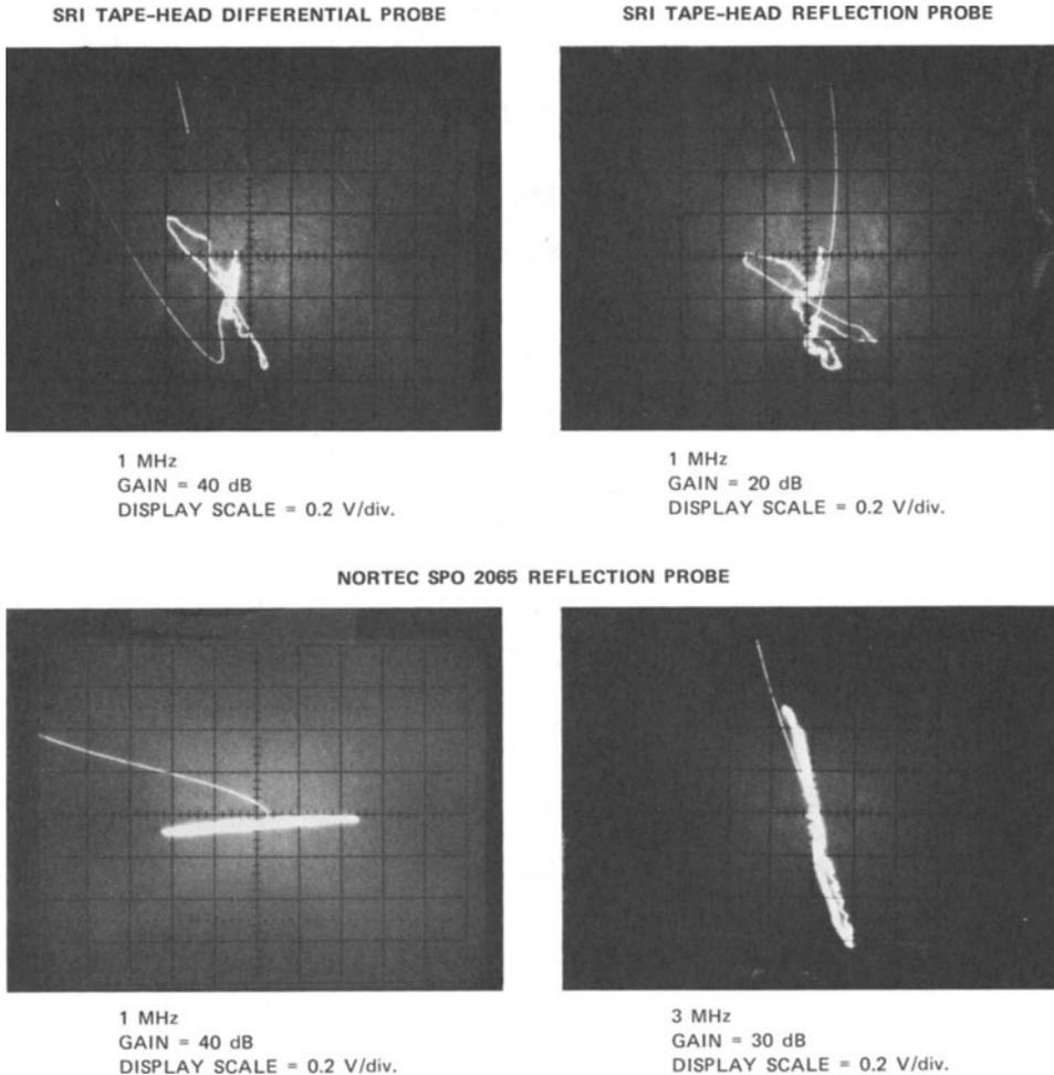
(Material: titanium alloy; crack length: 0.030 in.)
