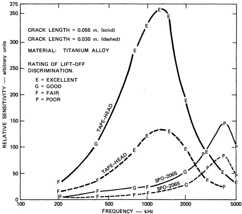
Fig. 4. Reflection-probe frequency responses.
