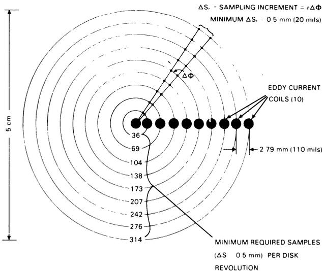
Fig. 3. Curvilinear eddy current imaging disk and coil array.
