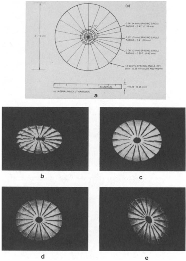
Fig. 5. Eddy current resolution test block and associated images: a) test block of simulated radial cracks; b)-e) 3-D images of the radial slots using only 10 discrete coils.
