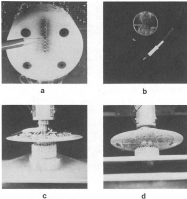
Fig. 2. Laboratory rotary eddy current scanning system: a) scanning head with 10 discrete coils; b) imaging coil and holder; c) and d) rotary disk and slip rings.
