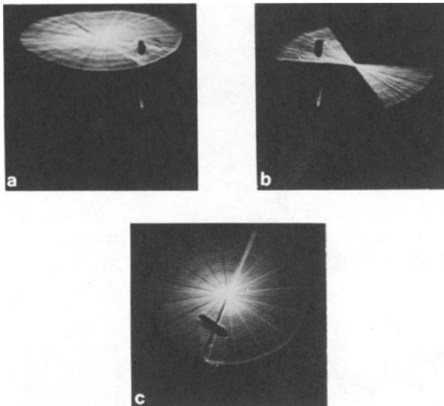
Fig. 9. Curvilinear scanned 3-D eddy current images of a fatigue crack simulating 50 discrete coils (i.e., 0.5 mm sampling).
