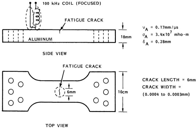
Fig. 6. Fatigue crack geometry in aluminum.
