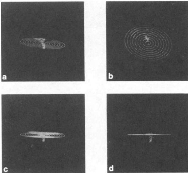
Fig. 8. Eddy current 3-D images of the fatigue crack using only 10 discrete coils (i.e., 2.5 mm sampling).
