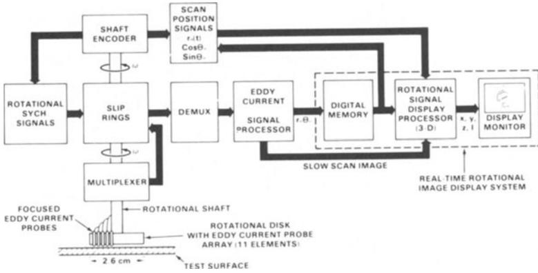
Fig. 1. Eddy current rotary scanner focused probe array imaging system.
