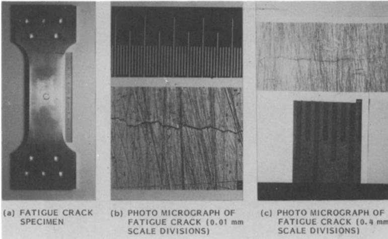
Fig. 7. Optical photographs of the fatigue crack in aluminum.
