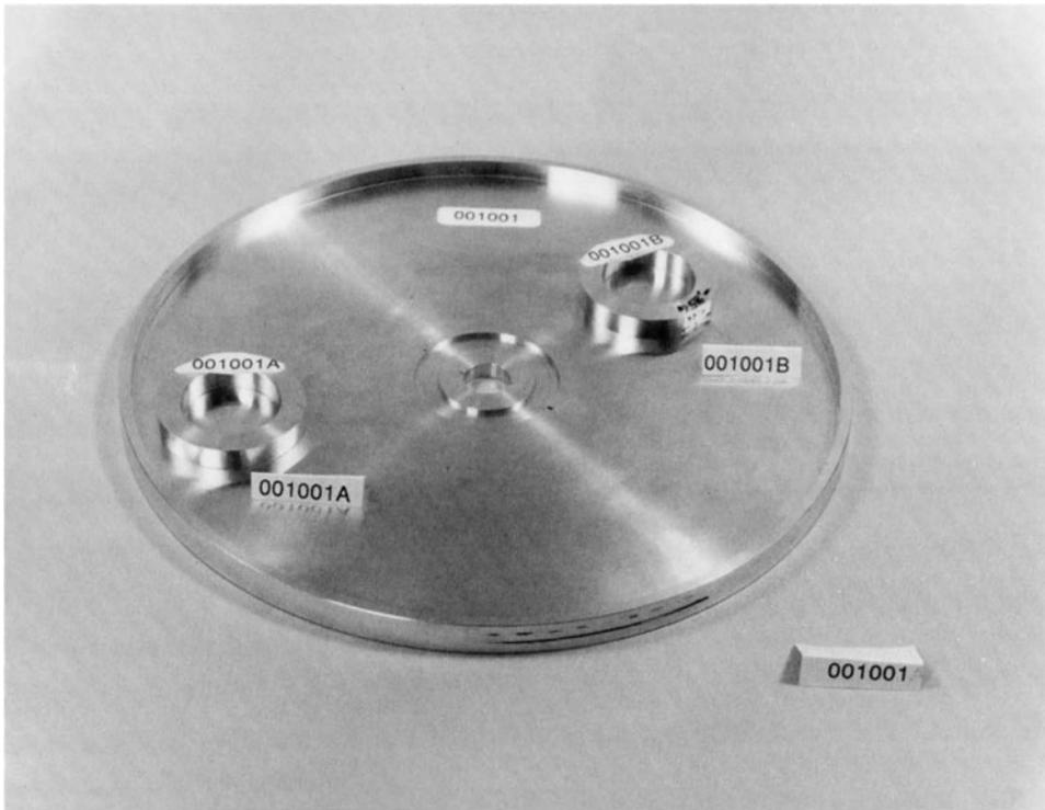
Fig. 1. CG disk test phantom, (PID #001001) with two of the three aluminum bushings (PID# 001001A and 001001B) laying on the disk.
