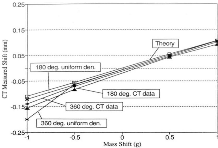
Fig. 4. Comparison of the shift in the CG for a mass shift in the test phantom including the curve for the theoretical shift.
