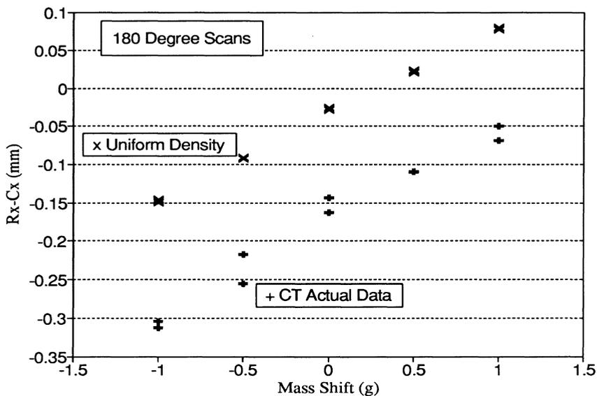
Fig. 2. Difference between center of geometry and CG for 180° scans.
