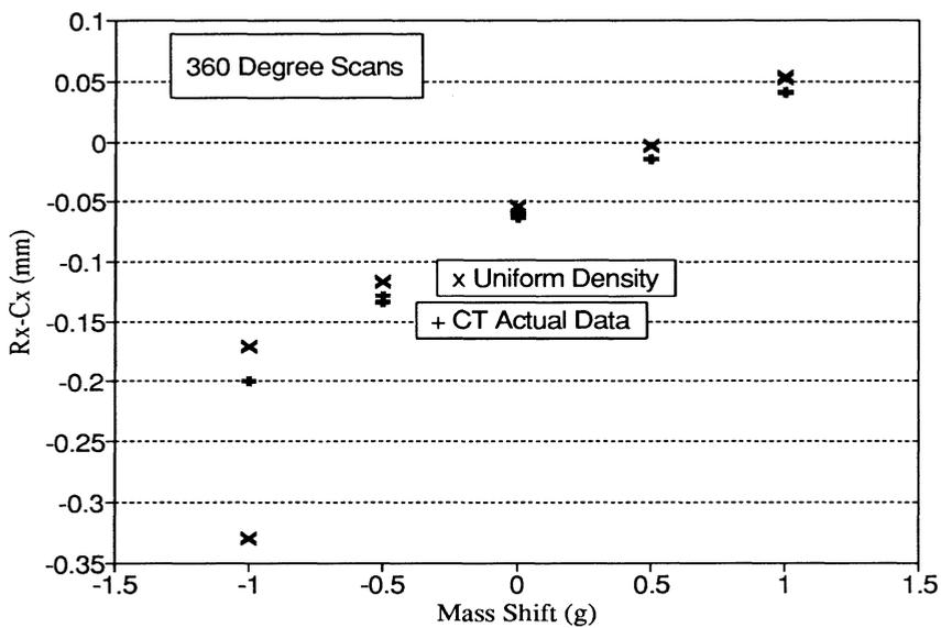
Fig. 3. Difference between center of geometry and CG for 360° scans.
