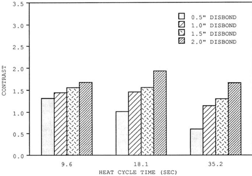
Figure 7. Contrast as a function of acquisition time and disbond width for impulse heating.
