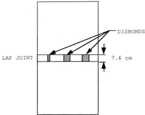
Figure 2. Typical sample configuration.
