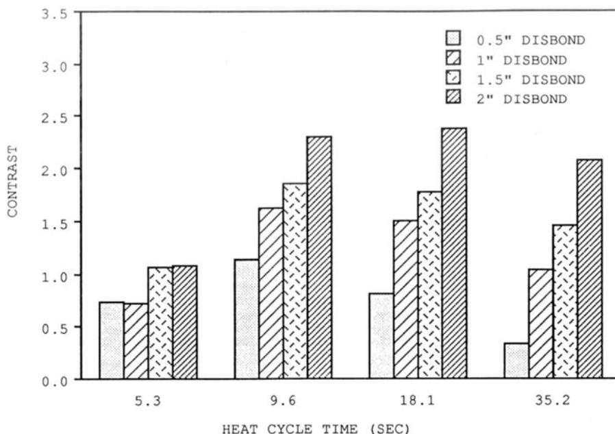
Figure 5. Contrast as a function of period time and disbond width for periodic heating.
