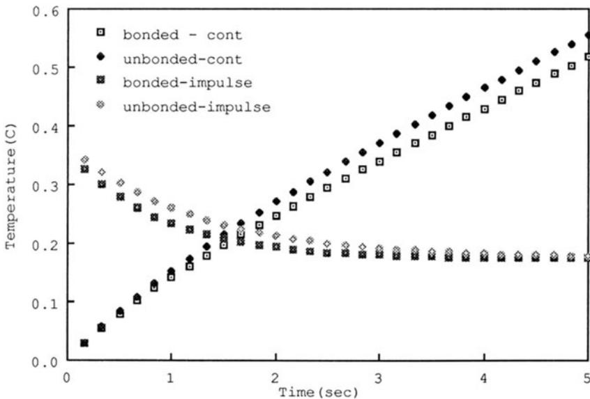
Figure 3. Thermal response of bonded and unbonded regions of lap joint to impulse and continuous heat flux.
