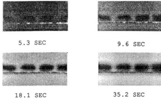
Figure 4. Time derivatives of IR images from cyclic heating of sample shown in figure 2. Period for heating cycle given under each image.
