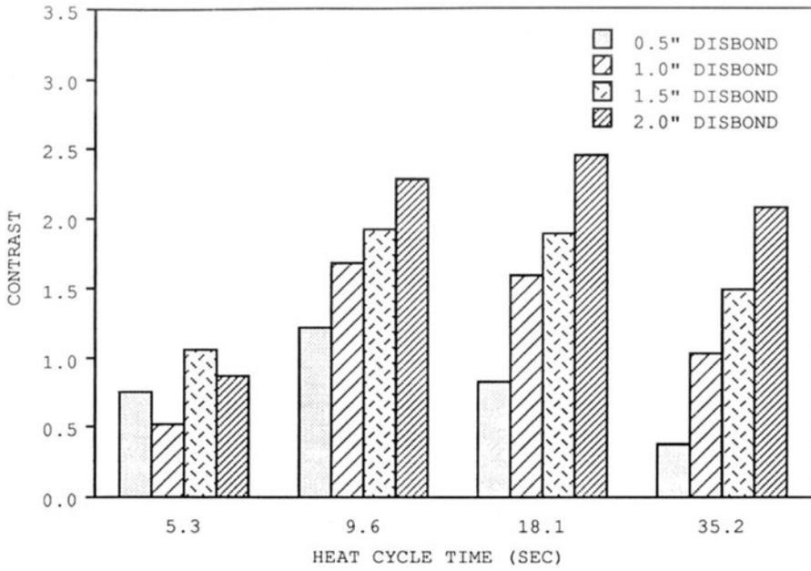
Figure 6. Contrast as a function of acquisition time and disbond width for pulse heating.
