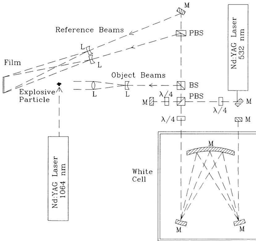
Figure 1. A schematic of the optical setup for high-speed dual exposure holography using a White cell as an optical delay line.
