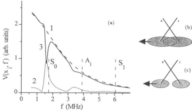
Figure 2: (a) Receiver voltage vs frequency for beam shift  $x_i = -10$  mm. Dashed curve (1) is specular component, dotted curve (2) is leaky wave, and solid curve (3) is total voltage. Reflection coefficient zeroes denoted by vertical dashed lines and labeled with mode designation. Schematic illustration of diffraction effects and beam overlap at low (b) and high (c) frequency for negative beam shift,  $x_i < 0$ .
