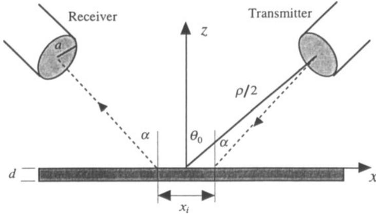
Figure 1: Schematic of experimental geometry for analysis of beam reflection from fluid-loaded structures; incident angle is  $\alpha$ ,  $\rho$  is the total water path, and  $x_i$  is the beam shift parameter. The plate is infinite in the  $y$  direction.
