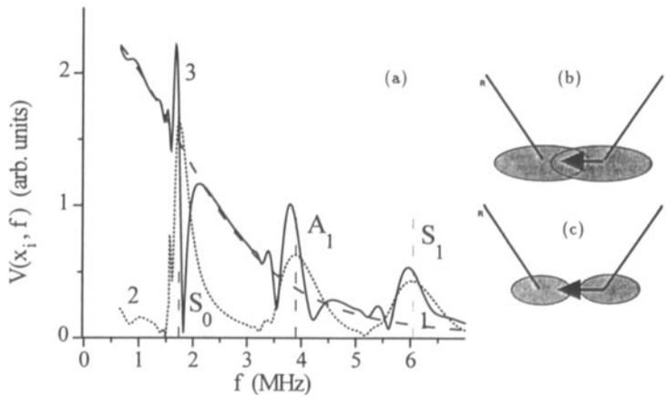
Figure 3: (a) Receiver voltage vs frequency for beam shift  $x_i = +12$  mm, showing the effect of diffraction on voltage minima. Dashed curve (1) is specular component, dotted curve (2) is leaky wave, and solid curve (3) is total voltage. Reflection coefficient zeroes denoted by vertical dashed lines and labeled with mode designation. Schematic illustration of diffraction effects and beam overlap at low (b) and high (c) frequency for positive beam shift,  $x_i > 0$ .
