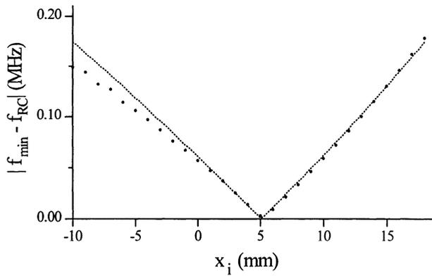
Figure 5: Absolute value of frequency difference  $f_{min} - f_{RC}$  between voltage minimum and corresponding RC zero for the  $S_0$  guided wave mode at an incident angle of  $\alpha = 25^\circ$ . Discrete points are the exact expression, and the curves are the approximate values;  $f_{min} < f_{RC}$  for values of  $x_i$  to the left of minimum.
