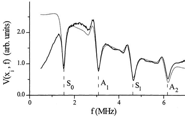
Figure 4: Experimental (solid curve) and theoretical (dotted curve) receiver voltage for a two-transducer frequency scan at  $\alpha = 20^\circ$  and  $x_i = +5$  mm. Reflection coefficient zeroes denoted by vertical dashed lines and labeled with mode designation.
