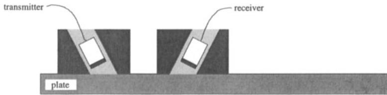
Figure 5. Schematic of set-up used for experimental verification of  $s_2$  mode
