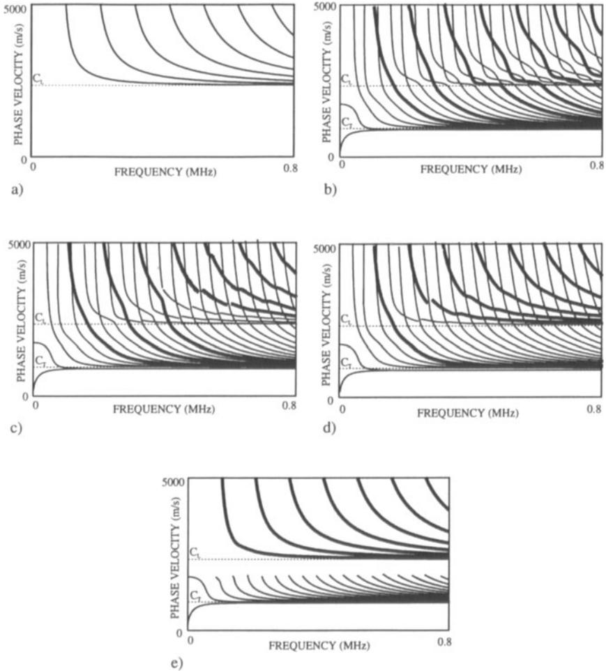
Figure 2. Dispersion curves for a) fluid-plate; b) zero attenuation; c) half attenuation ( $\alpha_L = 0.0275\text{Np/wavelength}$ ,  $\alpha_S = 0.143\text{Np/wavelength}$ ); d) full attenuation ( $\alpha_L = 0.055\text{Np/wavelength}$ ,  $\alpha_S = 0.286\text{Np/wavelength}$ ); e) four times attenuation ( $\alpha_L = 0.220\text{Np/wavelength}$ ,  $\alpha_S = 1.144\text{Np/wavelength}$ ). Longitudinal asymptotic modes shown in bold.
