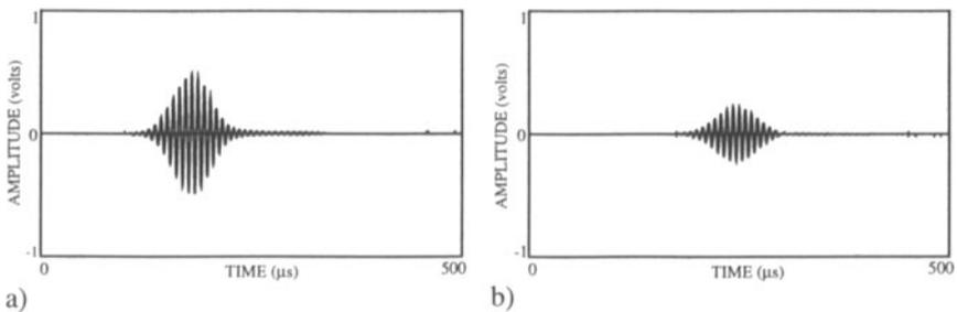
Figure 6. Time domain response of plate a) at first receiver position; b) at second receiver position.
