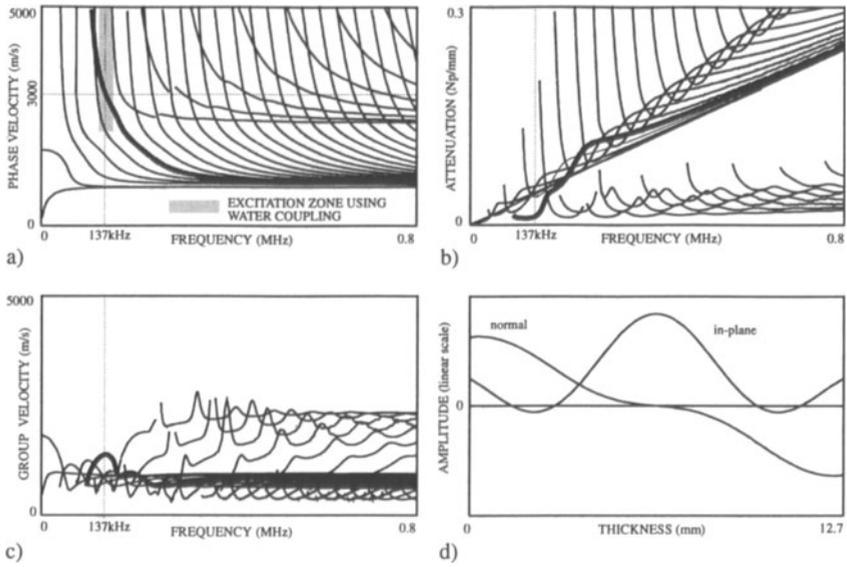
Figure 4. Dispersion curves for 12.7mm thick HPPE plate highlighting  $s_2$  mode. a) phase velocity; b) attenuation; c) group velocity; d) displacement mode shapes of  $s_2$  mode at 137kHz.
