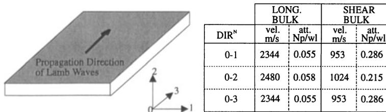
Figure 1. Bulk wave properties for high performance polyethylene
