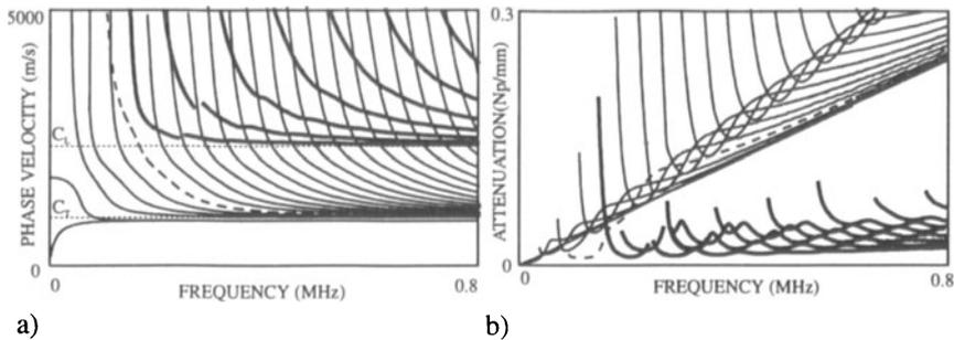
Figure 3. a) Phase velocity and, b) attenuation dispersion curves for the case of full attenuation ( $\alpha_L = 0.055\text{Np/wavelength}$ ,  $\alpha_S = 0.286\text{Np/wavelength}$ ). Longitudinal asymptotic modes shown in bold; longitudinal cut-off, shear asymptotic modes shown dotted.
