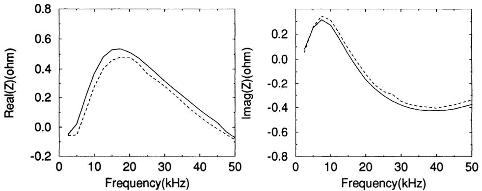
Fig. 2. Comparison of theoretical and experiment results. The left and the right pictures show the real and imaginary parts of the coil impedance change over a 1-mm 2024 aluminum plate with a flat hole on the bottom side. The experimental result is plotted with a dashed line and the theoretical result is plotted with a solid line. The threshold used is 0.05.
