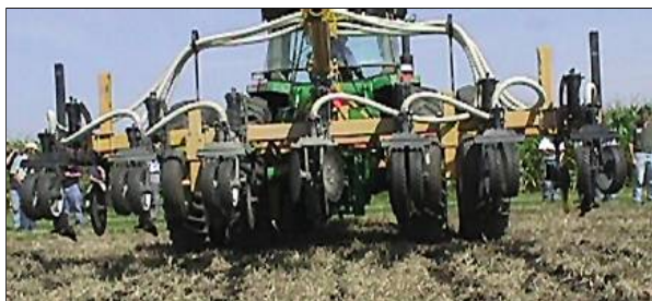
Above: Narrow knives on a drag hose applicator.
