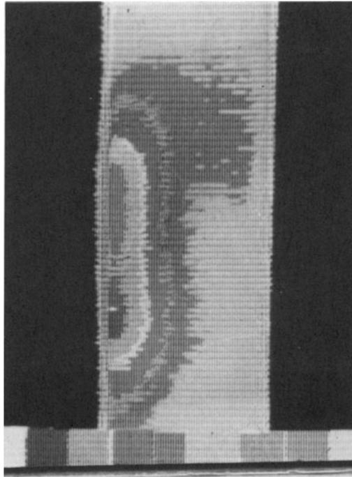
Figure 3. Vibrothermograph of composite edge delaminations.
