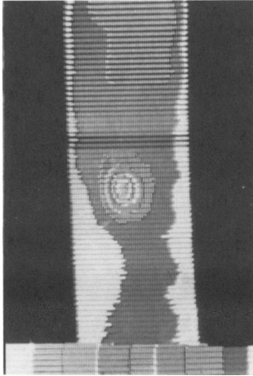
Figure 4. Vibrothermograph of composite with 1/5 in. (1.1 mm) square delamination (simulated by placing mylar square in specimen during fabrication).
