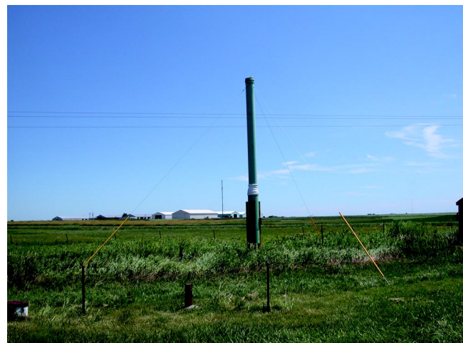
These soybean aphid suction traps in Boone County are composed of a 20-foot vertical tube with an electric fan at the base. The fan pulls air through the tube and deposits aphids into an alcohol-filled jar. (Matt O'Neal)
