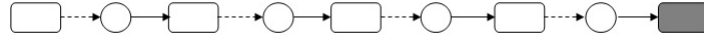
Figure 3.5 Chain of hold-and-wait dependencies while trying to acquire a lock leading to a deadlock.
