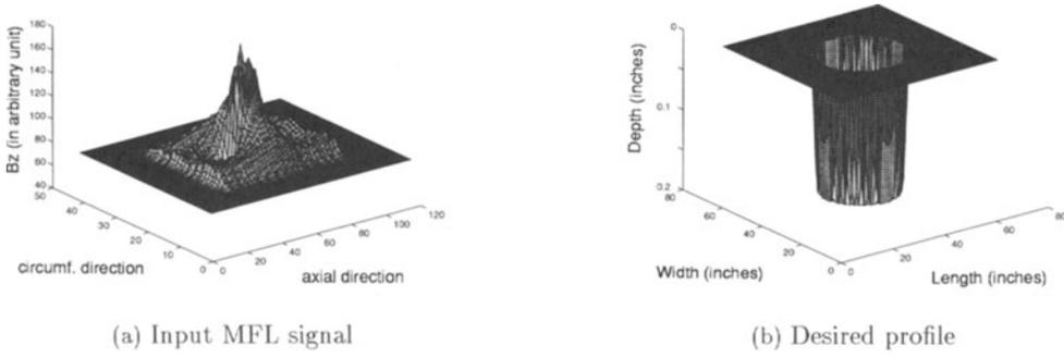
Figure 2: Mapping from an MFL signature to a defect profile.
