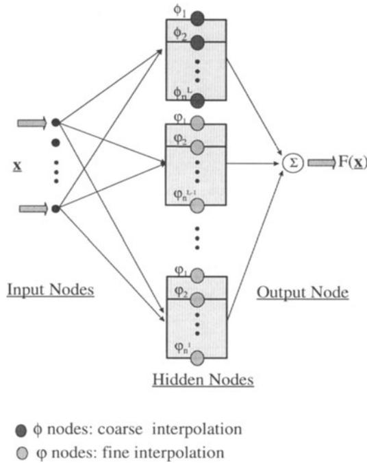
Figure 1: Architecture of a wavelet network.
