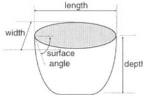
Figure 5: Geometry of defect profile.
