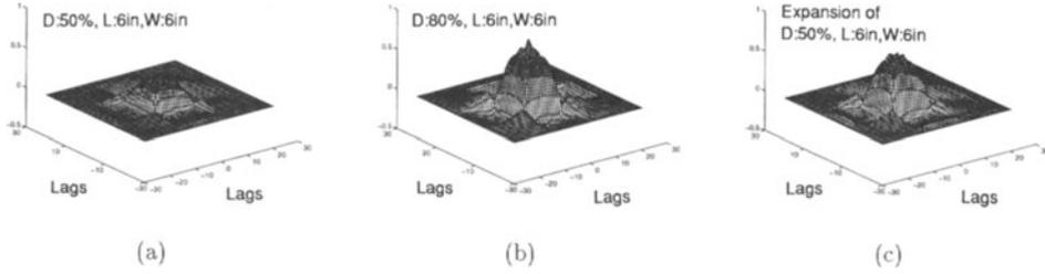
Figure 3: Illustration of the dyadic expansion (a) A typical covariance matrix of 50% depth MFL signal. (b) A typical covariance matrix of 80% depth MFL signal. (c) Expansion of the covariance matrix (a).
