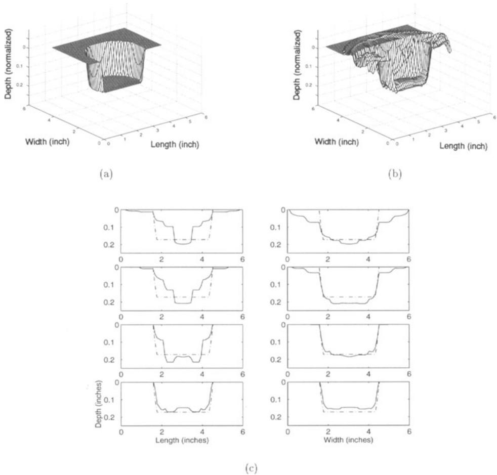
Figure 6: Comparison of true and predicted defect profiles (depth:50%,length:3in,width:3in). (a) True defect profile. (b) Predicted defect profile. (c) Effect of changing the number of resolutions (true profile: ---, predicted profile: —).
