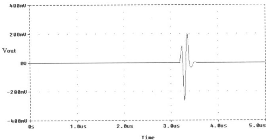
Figure 3 Pspice Simulation Result for PVDF Model, 30 Volt Excitation.
