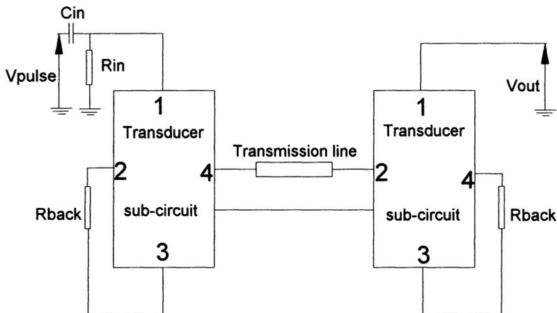
Figure 1 Through Transmission Pspice Simulation Circuit.
