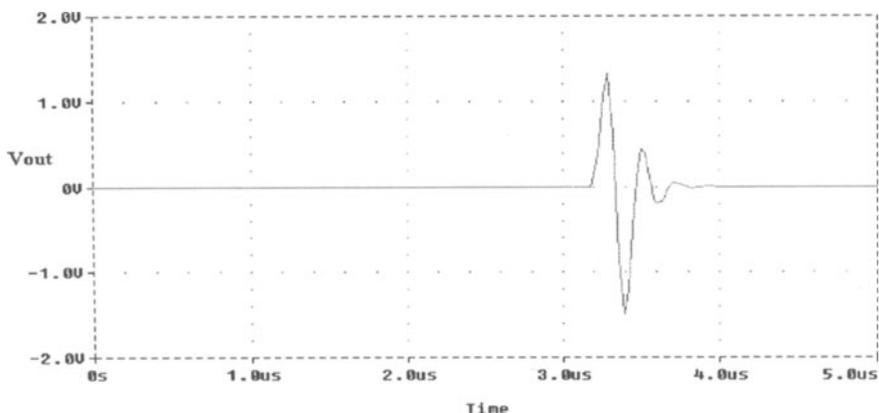
Figure 4 Pspice Simulation Result for PZT-5A, 30 Volt Excitation.
