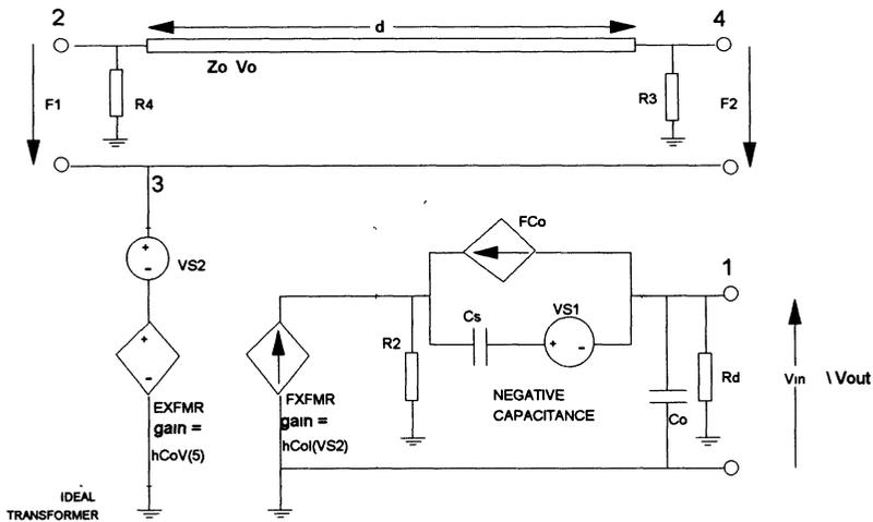
Figure 2 Equivalent transducer sub-circuit.
