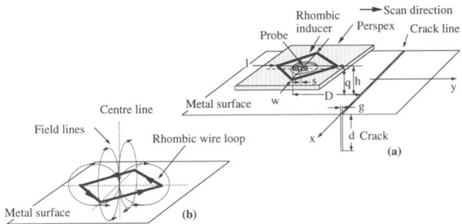
Fig. 1 (a) The schematic diagram of a rhombic wire loop and a linear probe attached below the long diagonal. The probe offset 's' is the distance between the short diagonal and the middle of the probe. (b) The field pattern of a high frequency current carrying rhombic inducer close to a metal surface.
