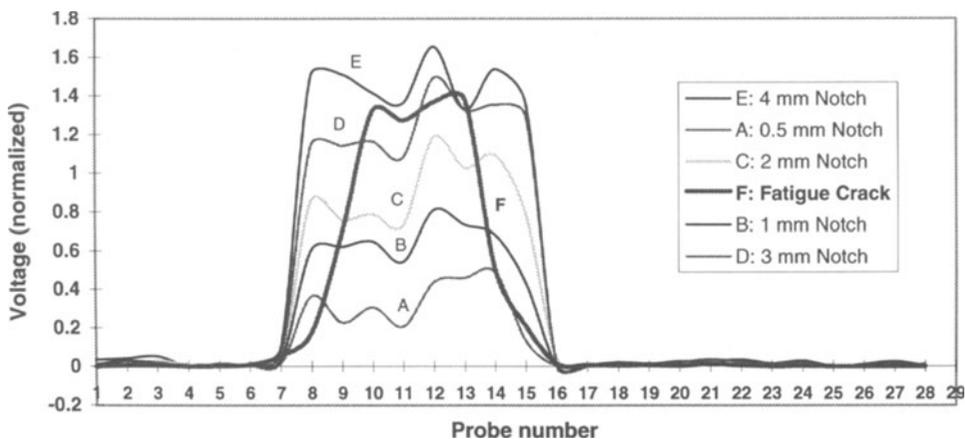
Fig.6 Results of the application of the array to a set of notches in a mild steel test-block and to a closed (invisible) fatigue crack in a mild steel block with the same width as the test block. In these experiments, the probes liftoff  $q = 0.83\ \text{mm}$ .
