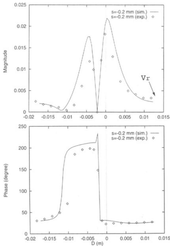
Fig.2 Magnitudes and phases of signals from the scan of a 4 mm deep saw-cut notch (with opening  $g = 150 \mu\text{m}$ ) in mild steel by the probe-inducer structure shown in Fig.1;  $w = 11.5 \text{ mm}$ ,  $l = 21.5 \text{ mm}$ ,  $h = 3.16 \text{ mm}$ ,  $q = 0.76$ ,  $s \approx -0.2 \text{ mm}$ , probe length = 4 mm, no. of probe turns = 80, probe layers = 2, probe core diameter = 0.88 mm, probe wire gauge = 0.0032" and  $f = 20 \text{ kHz}$ .
