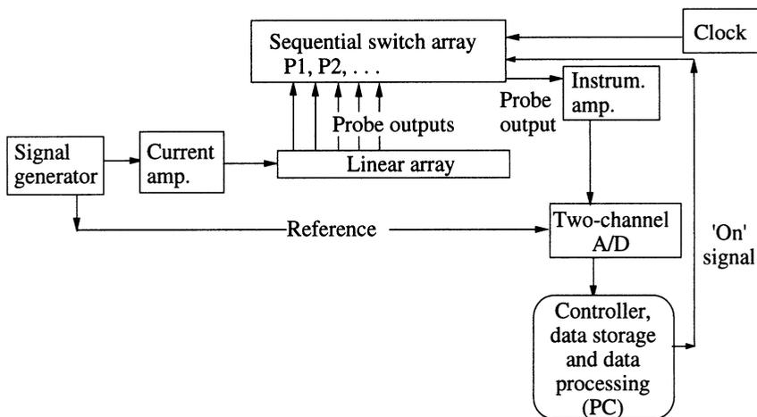
Fig.4 The block diagram of the detection system for the linear array.
