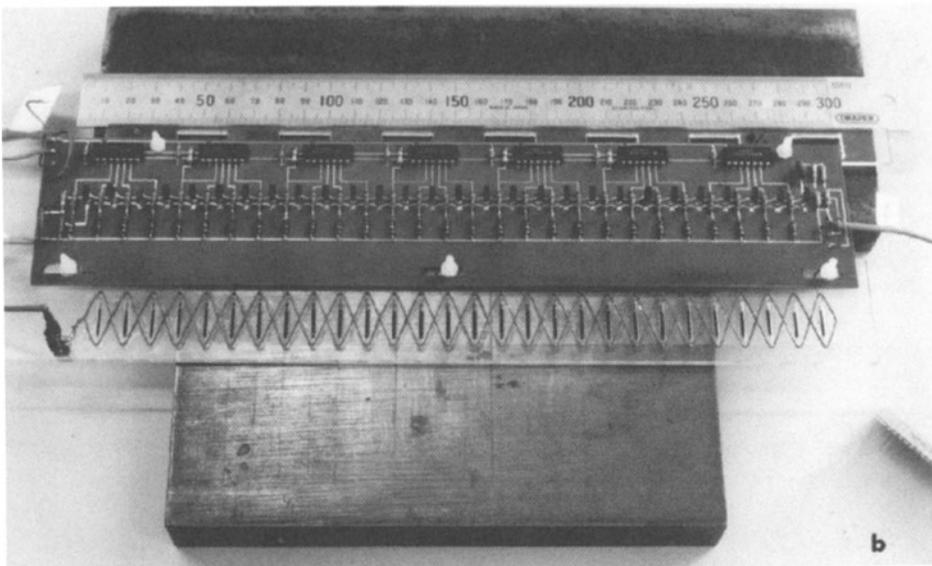
Fig.3 (a) The schematic diagram of a linear array using the rhombic inducer and the linear probe shown in Fig.1 and (b) the prototype 28 element array with the switching system.
