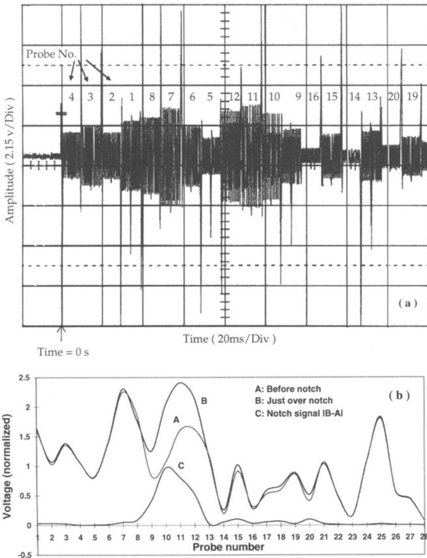
Fig.5 (a) The modulated signals (sinusoidal pulses) from the array in Fig.3.b when it was off and on the arc-circular notch and (b) the software demodulated signals (A and B) and the resultant (crack) signal (C). In this experiment, the probes liftoff  $q = 0.83$  mm.
