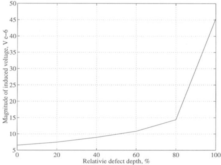
Fig. 2 Finite element simulation of the estimated magnitude of the induced voltage of the pickup coil as a function of the defect depth.
