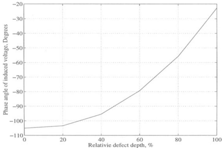
Fig. 3 Finite element simulation of the estimated phase angle of the induced voltage of the pickup coil as a function of the defect depth
