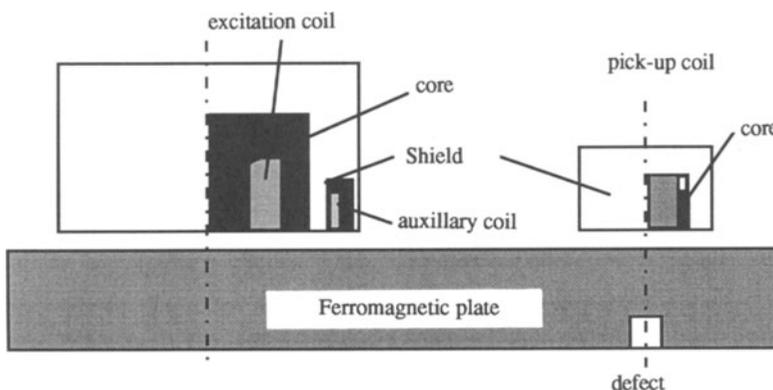
Fig. 1 Schematic of the RFEC probe for inspecting ferromagnetic flat plates
