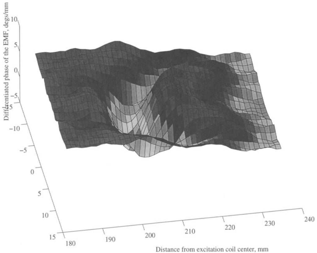
Fig. 6 Experimental data of for the slot machined in the 9.375 mm steel plate using a differential pickup coil sensor.
