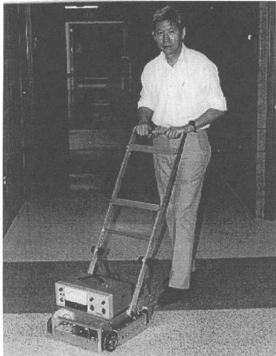
Fig. 4 A photograph of the RFEC probe with some of the instrumentation. Typically the system will be handled by the operator in the field.
