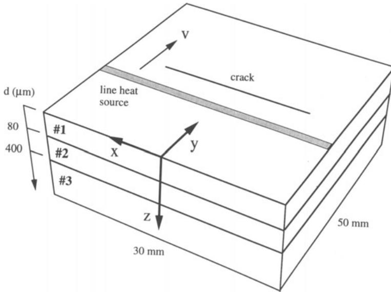
Fig. 1. A schematic drawing of the numerical model used in the calculations. The crack is parallel to the heating line.
