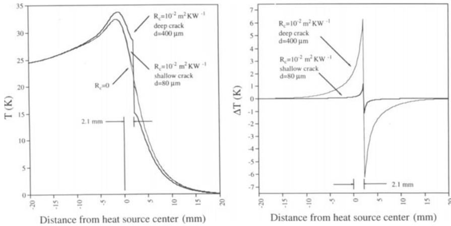
Fig. 2. a) The surface temperature profiles in the cases of a perfect sample, 80  $\mu\text{m}$  deep surface crack, and 400  $\mu\text{m}$  deep surface crack. b) The temperature difference profiles obtained by subtracting the curve with no defect from the curves with the cracks.
