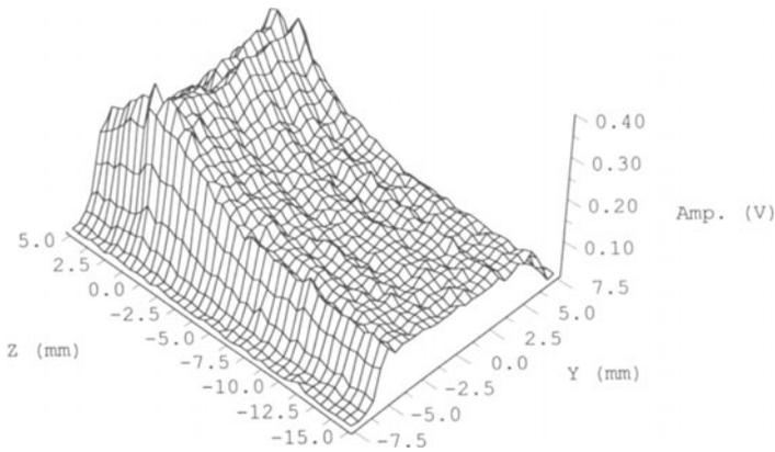
Fig. 5. Beam profile in Y-Z plane of 12-mm-wide transducer.
