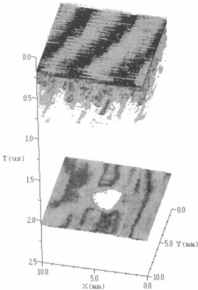
Fig. 10. Acoustic images of fiber orientation in the top surface and an artificial hole in the bottom surface of a unidirectional plate scanned by the 0.5-mm-wide transducer.
