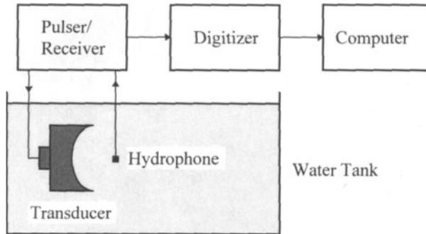
Fig. 2. Schematic of planar scanning setup.
