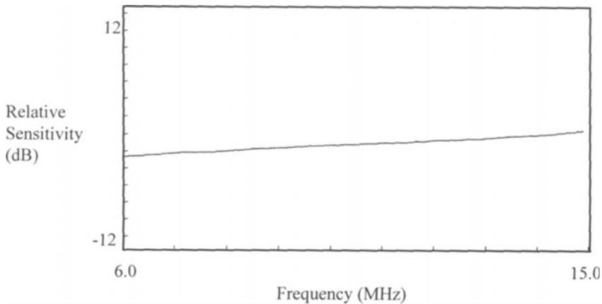
Fig. 3. Frequency response of the membrane hydrophone.
