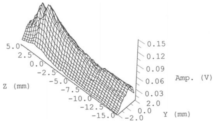
Fig. 7. Beam profile in Y-Z plane of 0.5-mm-wide transducer.
