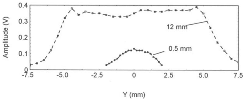
Fig. 8. Comparison of amplitude profiles in Y direction between 12 mm and 0.5 mm wide transducers.
