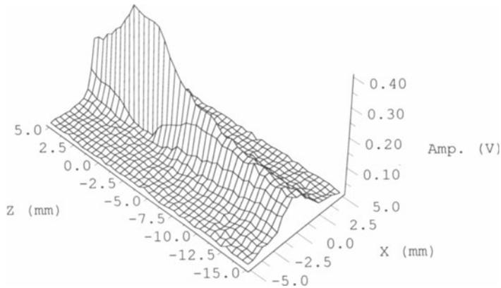
Fig. 4. Beam profile in X-Z plane of 12-mm-wide transducer.
