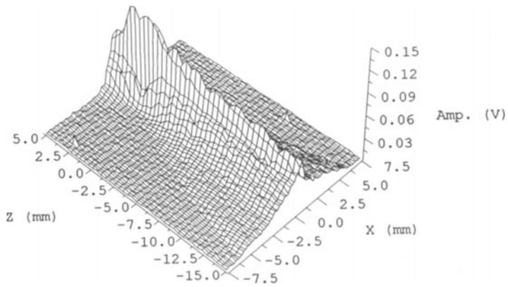
Fig. 6. Beam profile in X-Z plane of 0.5-mm-wide transducer.
