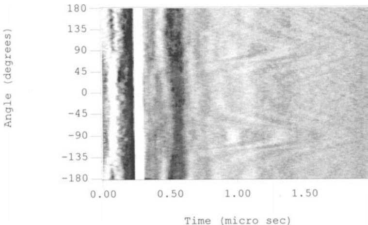
Fig. 9. Rotational scan of unidirectional composite using the 0.5-mm-wide transducer.
