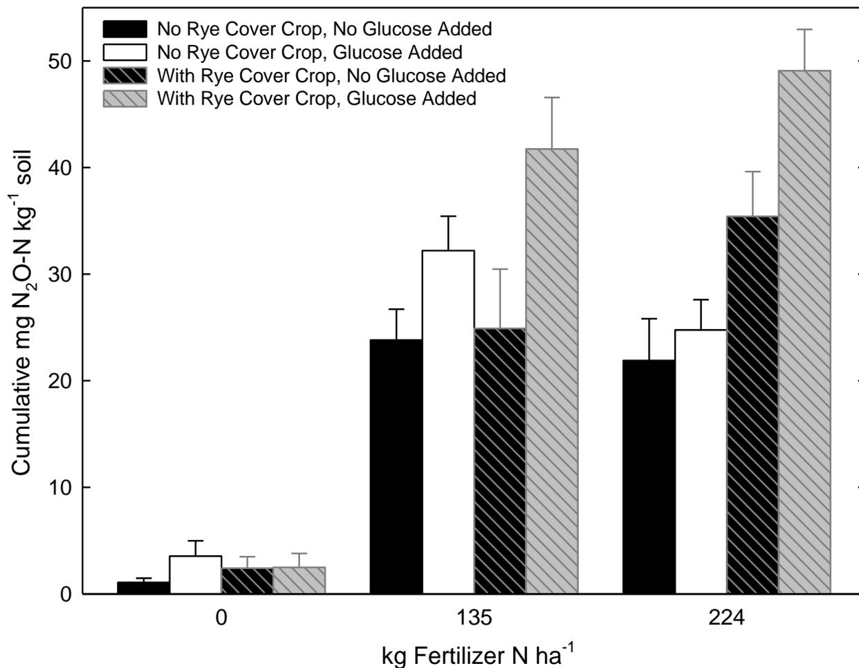
Figure 3.5. Cumulative  $\text{N}_2\text{O-N}$  emissions over 10 days from soils collected from the fertilizer bands of the field site and incubated at  $0.8 \text{ cm}^3 \text{ cm}^{-3}$  WFPS, showing the effect of glucose addition at each cover crop  $\times$  N fertilizer rate combination. Error bars show standard errors of means of 4 replicates.
