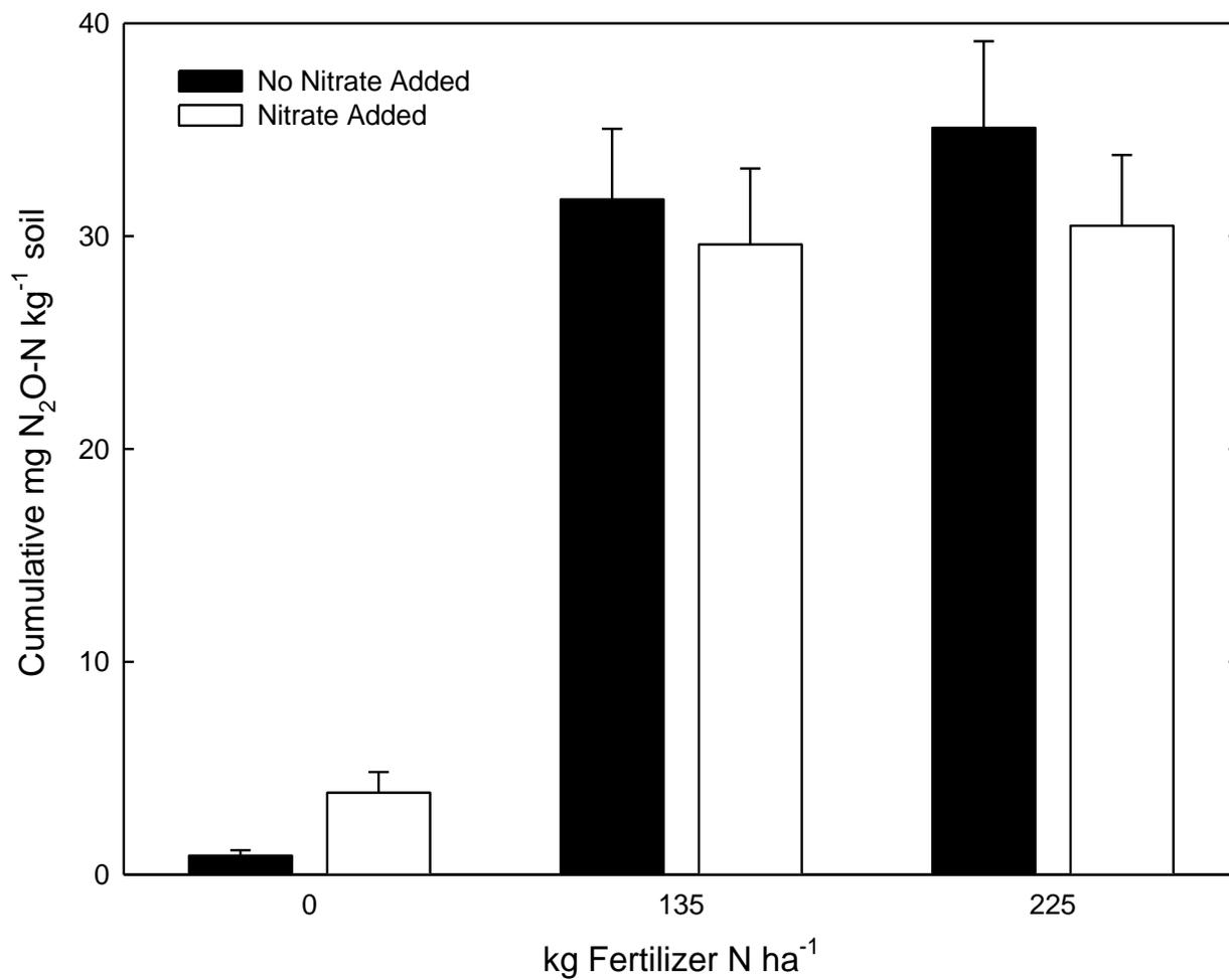
Figure 3.4. Cumulative N<sub>2</sub>O-N emissions over 10 days from soils collected from the fertilizer bands of the field site and incubated at 0.8 cm<sup>3</sup> cm<sup>-3</sup> WFPS, showing the effect of NO<sub>3</sub> addition at each N fertilizer rate across cover crop and glucose addition treatments. Error bars show standard errors of means of 4 replicates.
