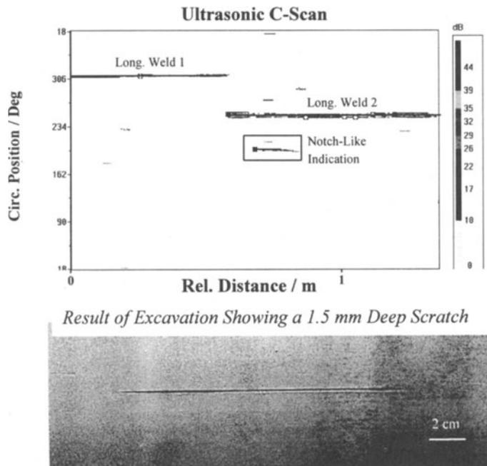
Figure 4. Top: C-scan of a pipe joint from a 26" crude oil line indicating an external notch-like defect. Bottom: Results of the verification excavation show a 160 mm long, 1.5 mm (18 % WT) deep groove.
