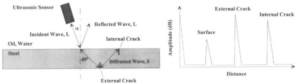
Figure 1. Measuring geometry (left) and corresponding A-scan (right).
