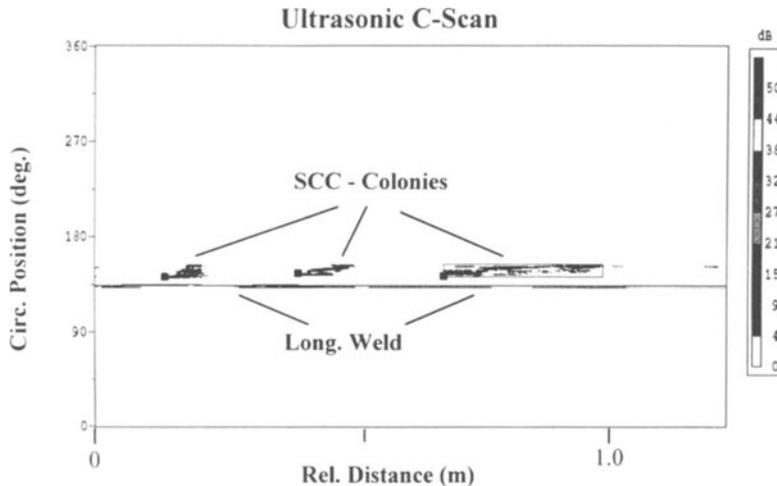
Figure 5. C-scan of a 56" pipe joint showing three SCC-colonies adjacent to the longitudinal weld.
