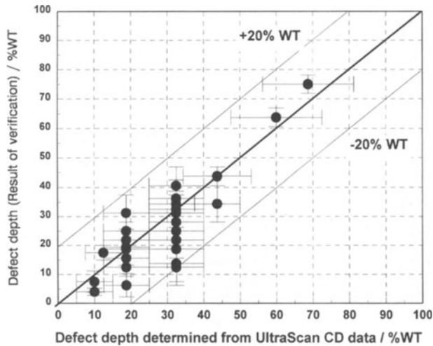
Figure 7. Comparison of crack depth determined from UltraScan CD data with verification results (from 40 excavations)
