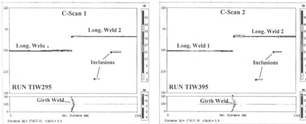
Figure 3. Comparison of C-scans from the same pipe joint recorded during two separate runs (26" crude oil pipeline). The C-scans at the bottom show the results of the wall thickness sensors indicating the location of the girth weld.
