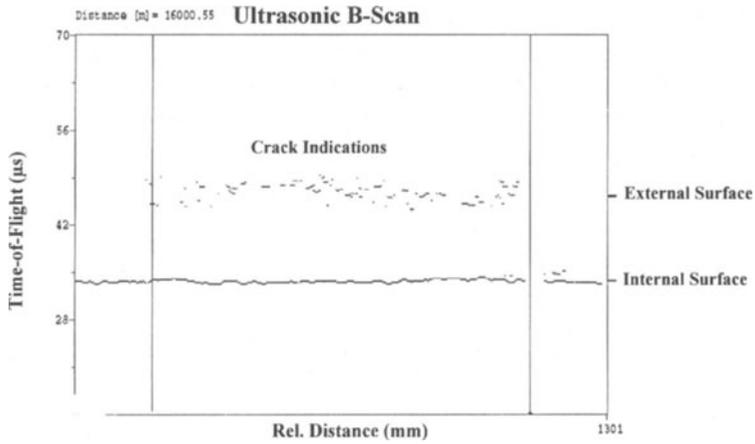
Figure 6. B-scan showing crack indications from part of a SCC colony at the external side of a 56" pipe joint. Here, the crack lengths are below 30 mm, the estimated depths are up to 3 mm.
