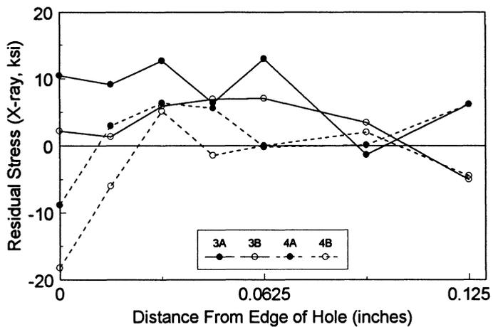
Figure 9 Measurements around two holes with approximately zero residual stress.
