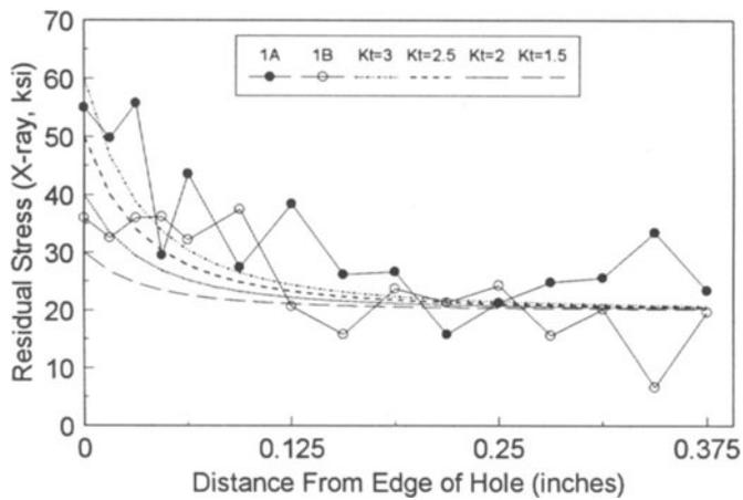
Figure 8 Measurements around a hole with tensile residual stress.
