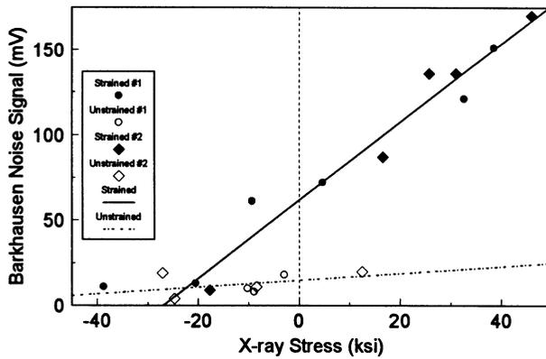
Figure 3 Calibration of BNA measurement against X-ray measurement.
