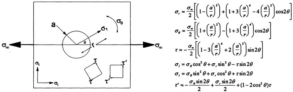
Figure 5 Terms and stress concentrations around a hole under applied load.
