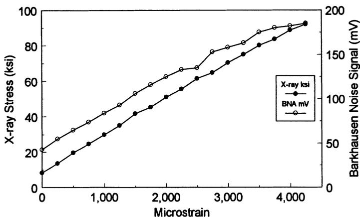
Figure 1. X-ray and Barkhausen noise measurements on four point bend sample.
