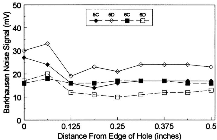
Figure 11 Longitudinal data around two holes with compressive residual stress.
