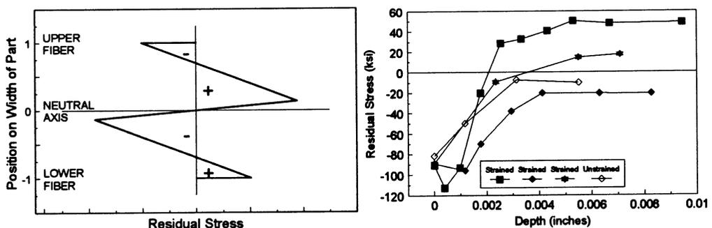
Figure 2 Width and depth variation of residual stress.
