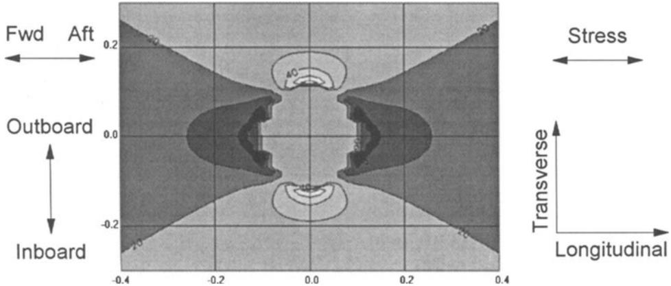
Figure 6 Calculated stress concentrations around a hole for an applied load of 20 ksi.
