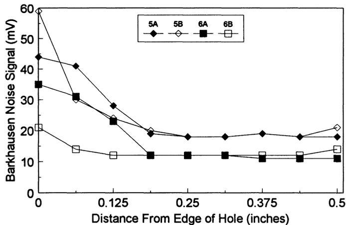
Figure 10 Transverse data around two holes with compressive residual stress.
