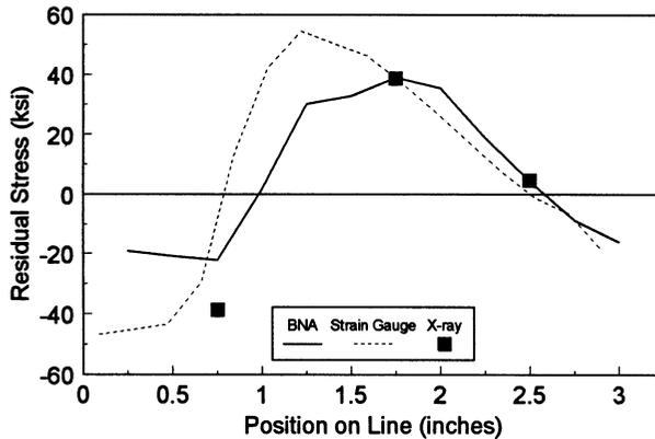
Figure 4 Check of measurement by X-ray, Barkhausen noise and strain gauge.
