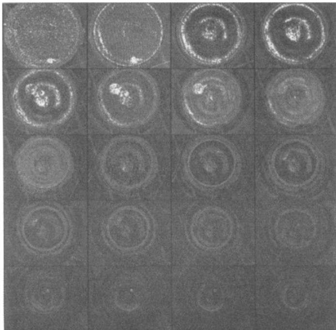
Figure 6. Montage of amplitude C-scans from Boeing Composite Repair Panel 3, with increasing depth left to right, top to bottom. Scan size 28.3 cm x 22.0 cm; step size 0.1 cm.
