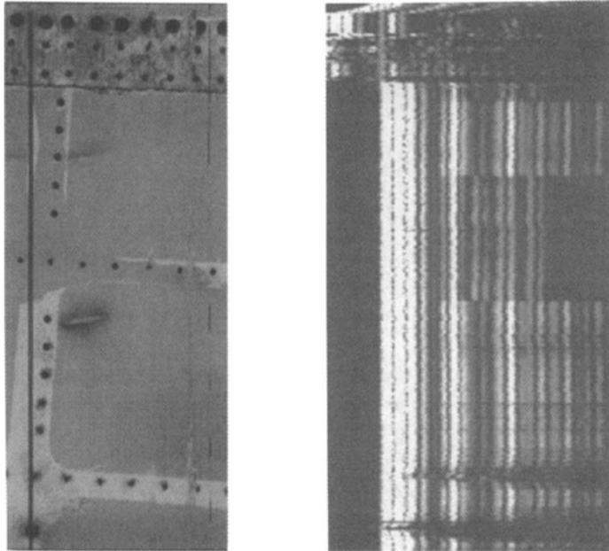
Figure 4. Peak amplitude C-scan (left) and B-scan image from Boeing 737 testbed at BS 887 S20-22R, behind rear cargo door. Location of B-scan is indicated in the C-scan image by double lines. Transducer: 15 MHz, 0.5" dia., 2.0" focus (water); scan size 55 x 22 cm; stepsize: 1 mm.
