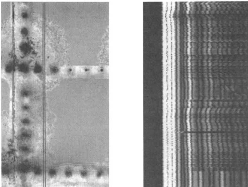
Figure 5. Peak amplitude (left) C-scan and B-scan images of fuselage skin back surface echo on Boeing 737 testbed at BS 887 S23-24R, behind rear cargo door. Location of B-scan is indicated in the C-scan image by double lines. Transducer: 15 MHz, 0.5" dia., 2.0" focus (water); scan size 39 x 22 cm; stepsize: 1 mm.
