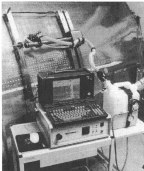
Figure 1. Dripless Bubbler Ultrasonic Scanning System.
