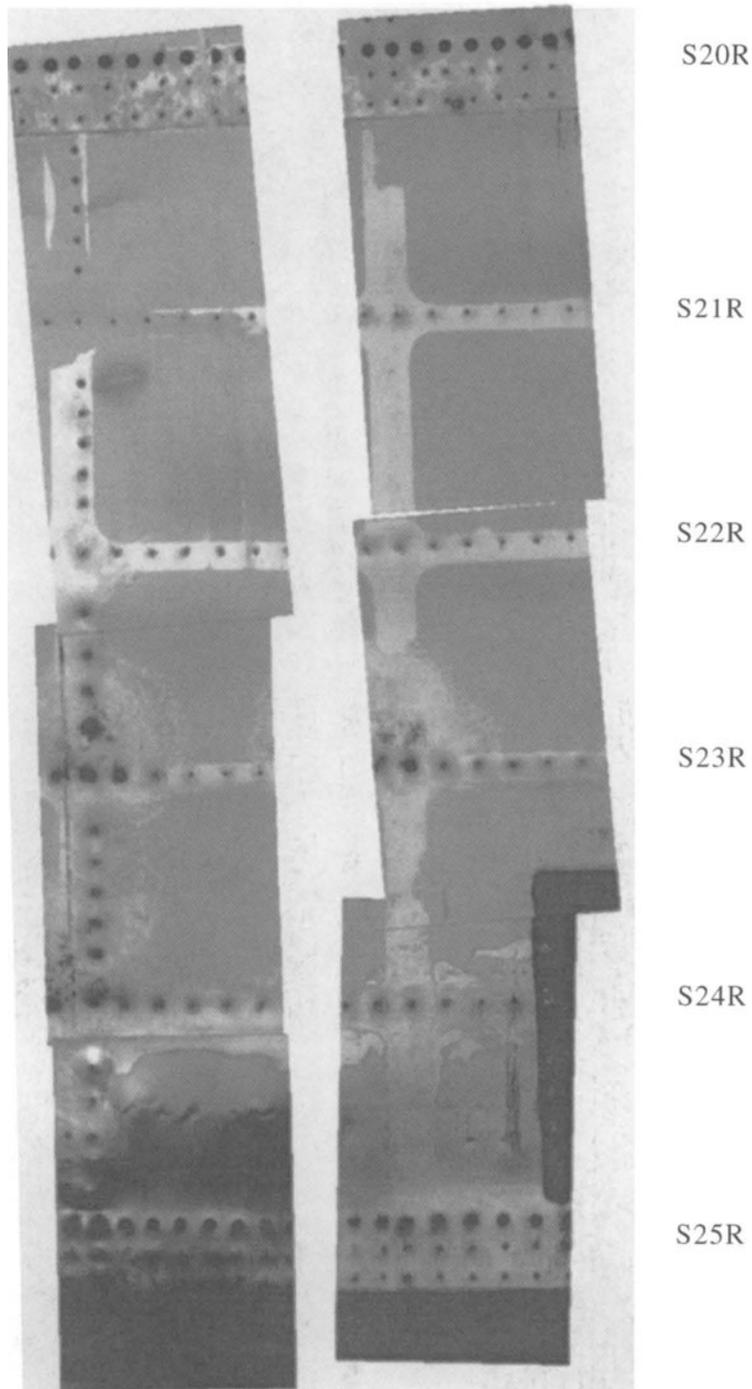
Figure 3. Composite of back surface echo C-scan peak amplitude images, showing corrosion and disbonds in the region behind the rear cargo door, at BS887-877 S20-25R, of the FAA-AANC Boeing 737 testbed (Sample 100). For all scans, transducer: 15 MHz, 0.5" dia., 2.0" focus; step size: 1 mm.
