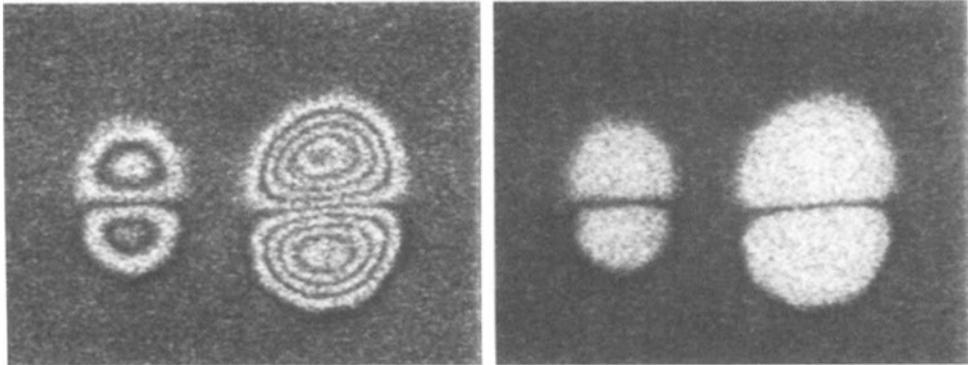
**Figure 1. Typical shearography results show the exact size shape and location of the defect, either with fringes (left), which show a quantitative measure of strain, or without fringes (right) showing an easily detectable indication.**
