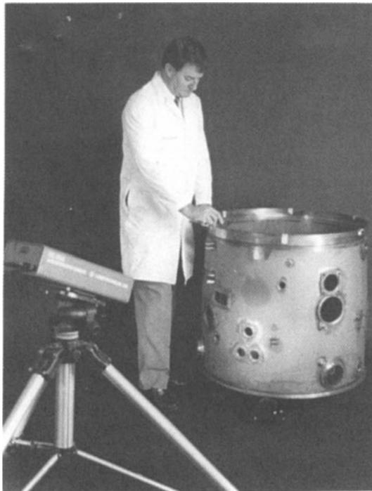
**Figure 2. F100 Fan Duct, 32 inches in diameter, 28 inches high and approximately 0.3 inches thick. Titanium skins over titanium honeycomb. Tested using LTI-4000 series Shearography system with vibration excitation between 4 and 10kHz.**
