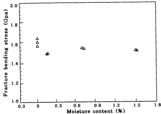
Fig. 6 Relation between fracture bending stress and moisture content
