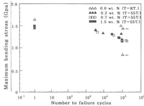
Fig.7 Residual fatigue bending strength variations according to moisture absorption contents
