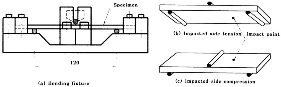
Fig. 1 Specimen supporting fixture for three-point bending test.
