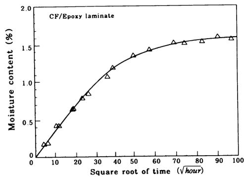
Fig. 3 Moisture content as a function of time under hygrothermals
