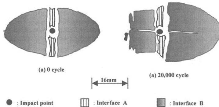
Fig.4 Progressive damage during fatigue bending test when the impacted side is compressed
