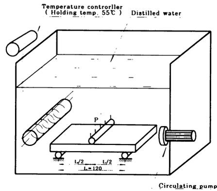
Fig. 2 Test arrangement of three-point bending fatigue test under water
