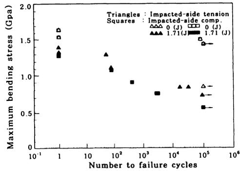
Fig. 5 Residual fatigue bending strength of damaged specimen
