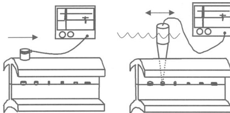
Figure 3. Contact and immersion testing of I-beam specimen.
