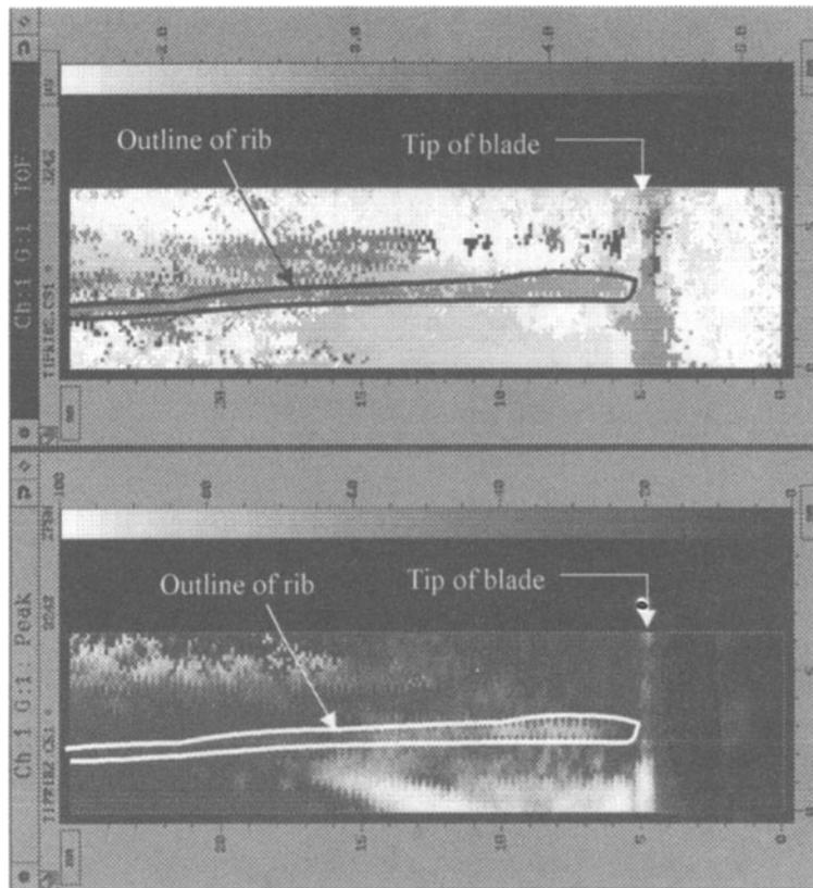
Figure 10. Time of flight C-scan (top) and amplitude C-scan (bottom). High amplitude (lighter gray) in amplitude C-scan indicates lack of bond.
