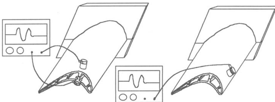
Figure 8. Through transmission (left) and pulse echo testing of bonded blade.
