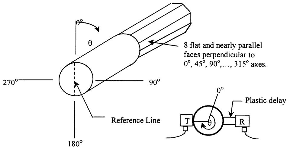
Figure 1. Method for measuring longitudinal wave velocities in CMSX-4 single crystal sample.
