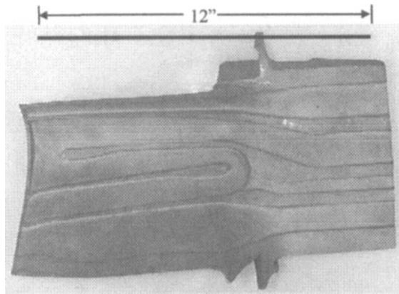
Figure 7. Convex half of blade prior to bonding.
