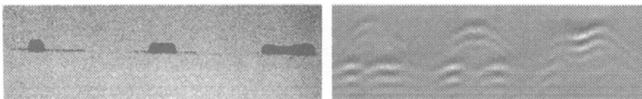
Figure 4. Micrograph (left) and B-scan of three slot defects ( $1/32''$ ,  $1/16''$ ,  $1/8''$ ) and disbond at bondline.
