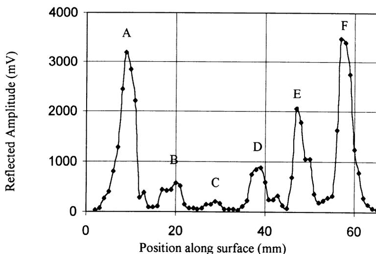
Figure 5. Results on I-beam specimen in contact mode.
