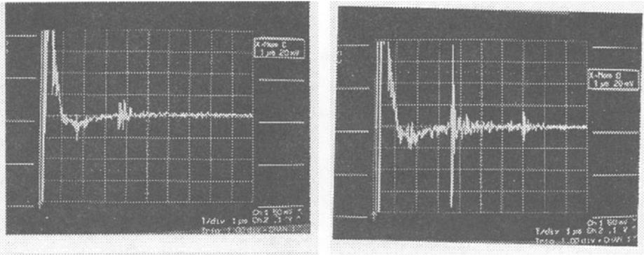
Figure 9. Low reflectivity of a good region of the bond (left) and high reflectivity of a poor region of the bond (right).
