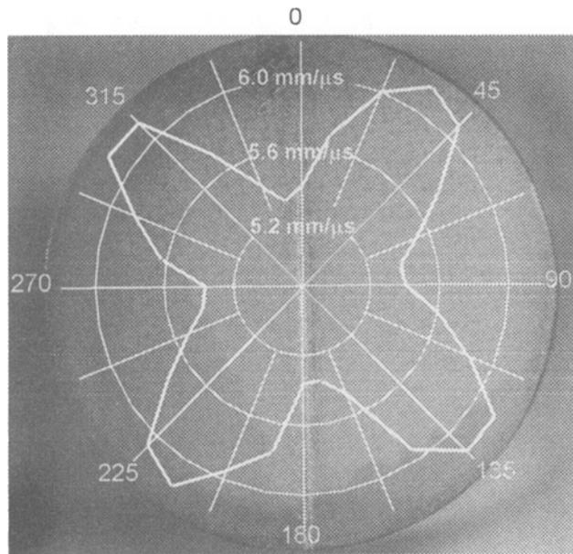
Figure 2. Longitudinal Velocity ( $\text{mm}/\mu\text{s}$ ) vs. angle from reference line (degrees) superimposed on a micrograph of the etched end of specimen.
