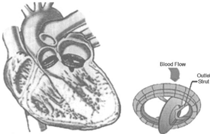
Figure 1. Prosthetic heart valve. A single leg separation occurs in the outlet strut.
