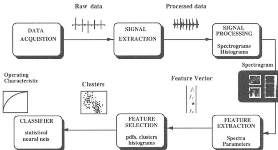
Figure 2. Classification protocol used for heart valve condition determination
