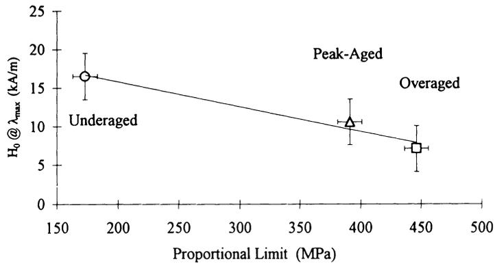
Figure 4. Magnetic fields  $H_0$  of low-field peaks in Figure 3(c) vs. the proportional limits of the underaged (o), peak-aged ( $\Delta$ ), and overaged ( $\square$ ) A710 steel samples.
