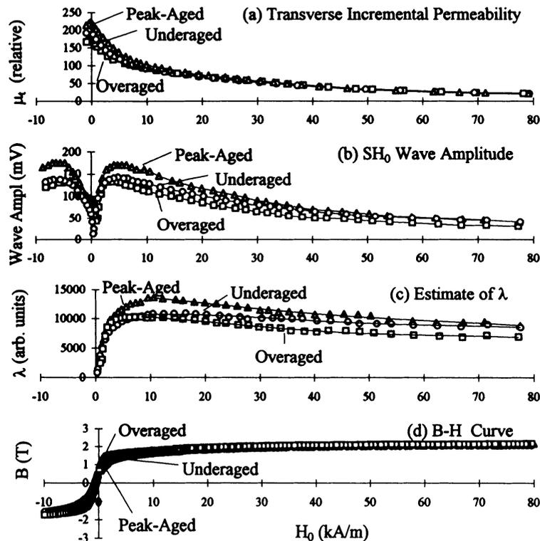
Figure 3. (a) Transverse incremental permeabilities, (b)  $SH_0$  wave amplitudes, (c) estimates of  $\lambda$  from Equation (3), and (d) B-H curves obtained in the underaged (o), peak-aged ( $\Delta$ ), and overaged ( $\square$ ) A710 steel samples.
