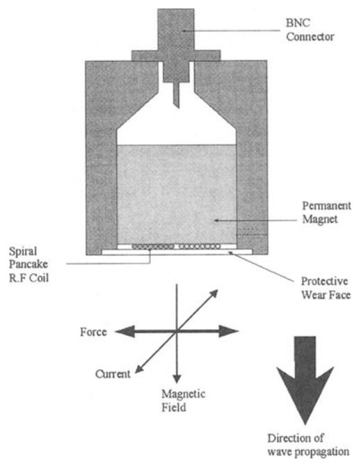
Figure 2. Schematic of EMAT showing field vectors
