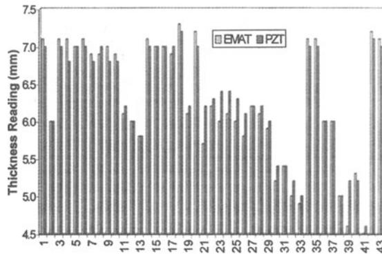
Figure 6. Comparison of EMAT and Piezoelectric Thickness Measurements
