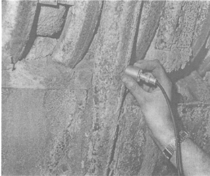
Figure 4. Typical conditions for EMAT tests on boiler tubes
