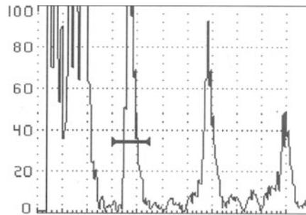
Figure 5. Typical EMAT waveform, the gate on the Ultrasonic Flaw Detector is set on the first backwall echo
