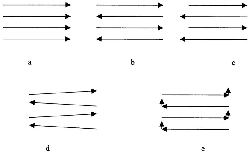
Figure 1. Magnetic Structures of a, ferromagnet, b, antiferromagnet, c, ferrimagnet, d, "canted" antiferromagnet and e, "d" resolved into ferromagnetic and antiferromagnetic components
