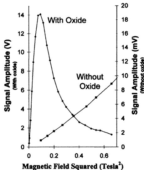
Figure 3. EMAT transduction efficiency as a function of magnetic bias field
