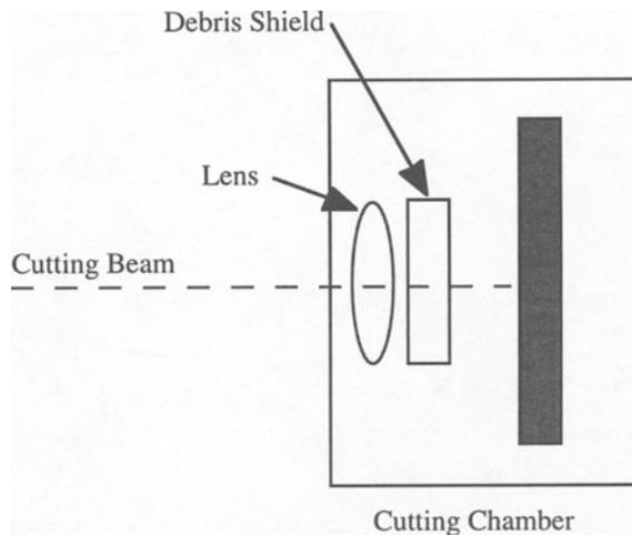
Figure 1. Laser cutting chamber.
