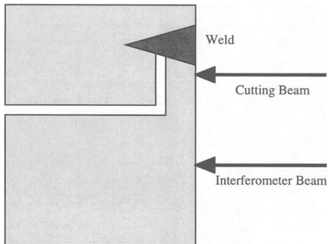
Figure 3. Welded part with step.
