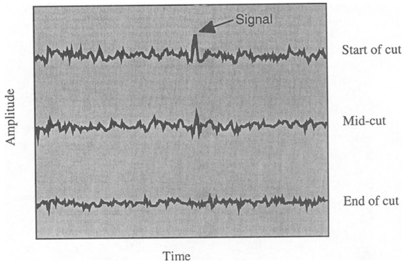
Figure 4. Signals detected from welded part with step.
