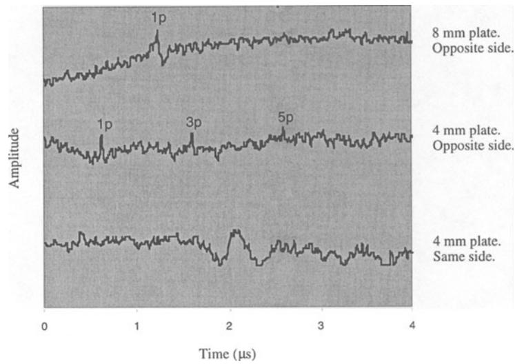
Figure 2. Signals detected from laser cutting on plates.
